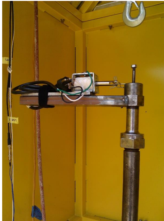
Figure 45: Shotgun shell solenoid-actuated ignition mechanism.
