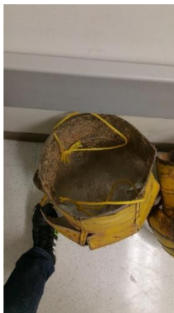
Figure 129: Steel oxygen tank/liner, which were destroyed during the experiment.
