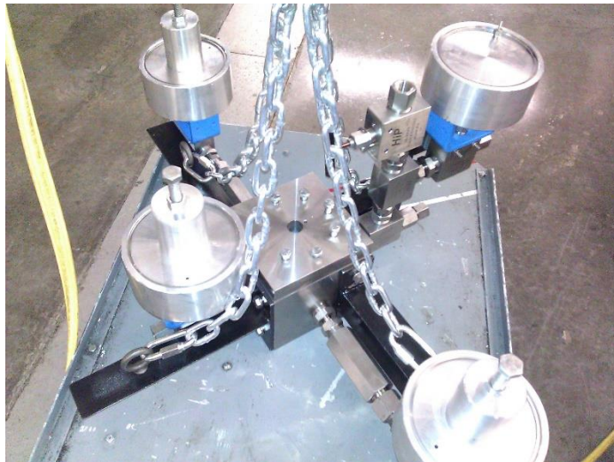
Figure 68: Newly fabricated and assembled gas manifold.
