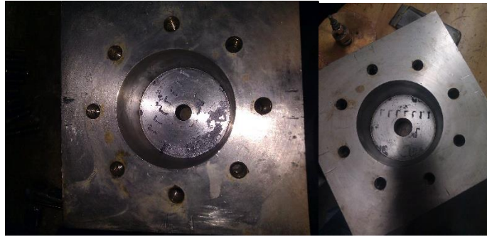
Figure 97: Gas manifold before and after additional boring process.
