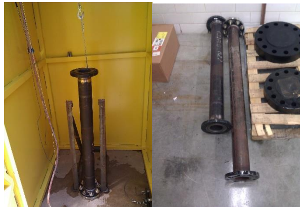
Figure 110: 3-ft-deep and 4-ft-deep shock tubes.
