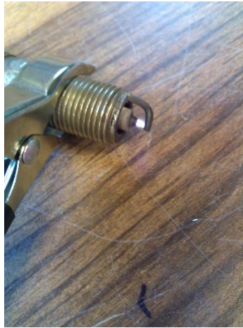
Figure 92: Brilliant arc for dimmer switch driven ignition circuit.
