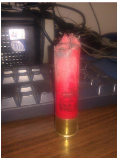
Figure 53: Reflected wave closed petals on the shotgun shell.
