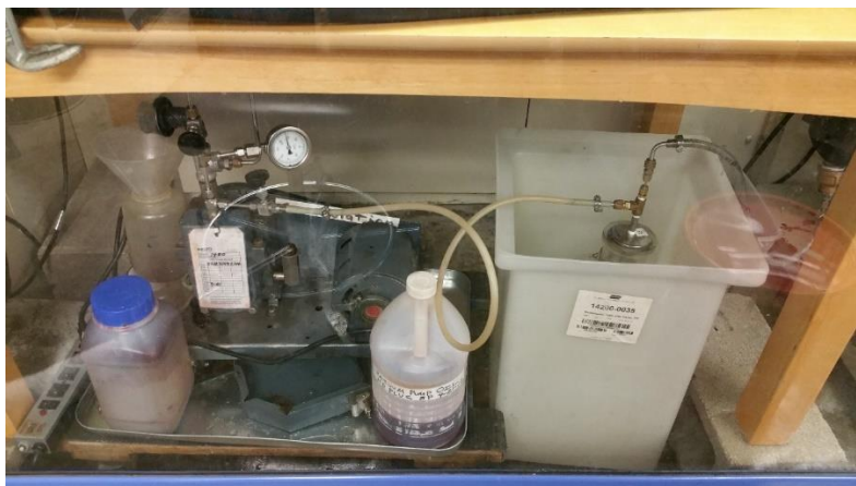
Figure 136: Vacuum pump and condensate collection vessel used for distillation.
