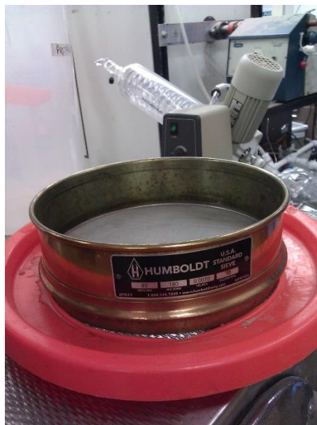
Figure 47: 80-mesh sieve tray used for recovering shock-treated biomass.
