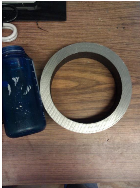
Figure 74: Cross-section of 8-in Schedule 160 pipe used for 20-L shock tube.
