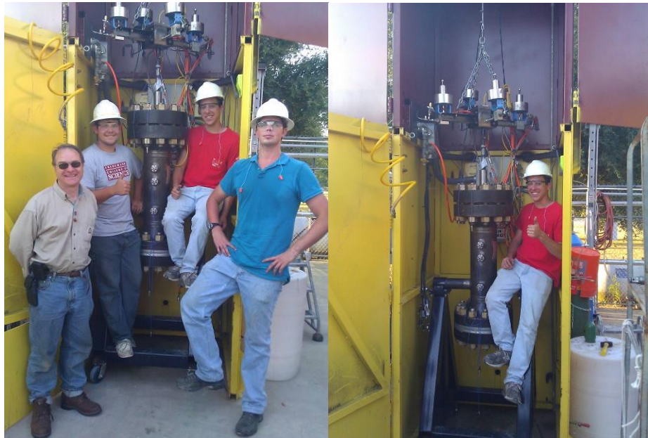
Figure 103: 20-L shock tube after first successful inaugural test.
