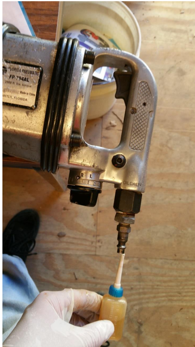
Figure F-1: Proper lubrication of impact wrench prior to EACH use.
