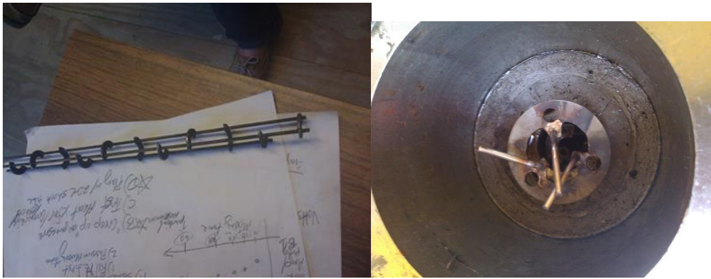
Figure 98: Roughness elements/baffles used to promote hydrogen detonation.
