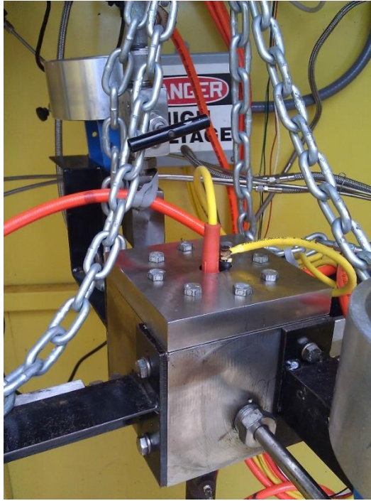
Figure 94: Gas manifold with glow plug adapter installed.
