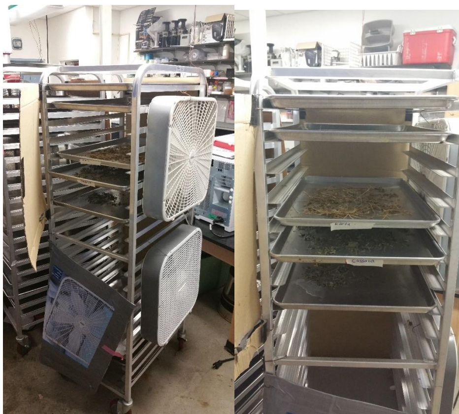
Figure C-1: Fan-driven drying racks.
