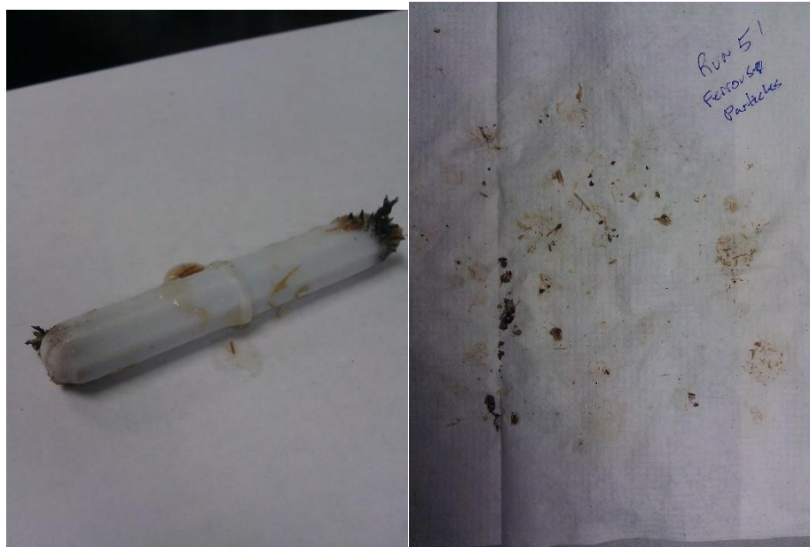
Figure 55: Ferrous particulate from shotgun shells and combine harvesting.
