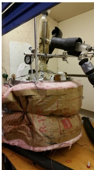
Figure 134: 22-L glass flask and vacuum distillation column with condenser.
