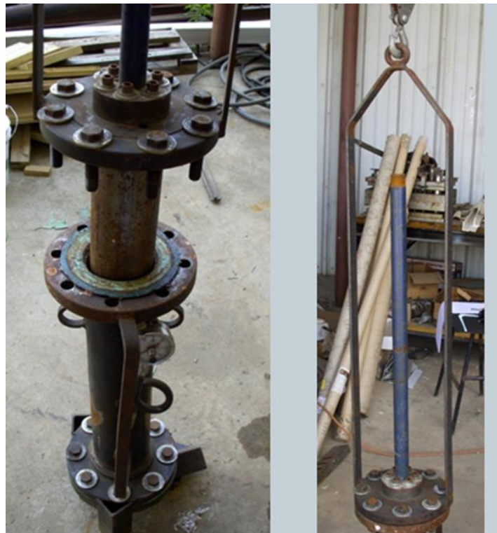
Figure 2: Shock tube prototype used for treating biomass.
