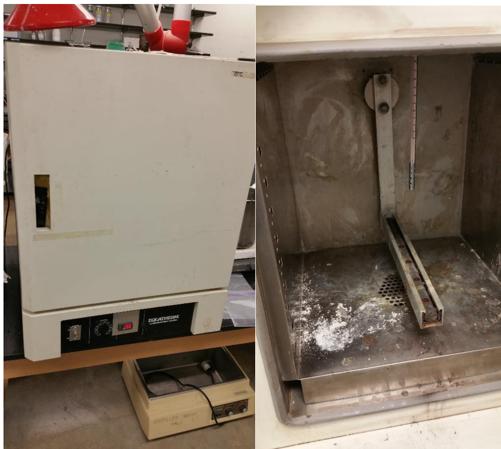
Figure 131: Oven with wrist-action shaker used for pipe bomb alkaline pretreatment.
