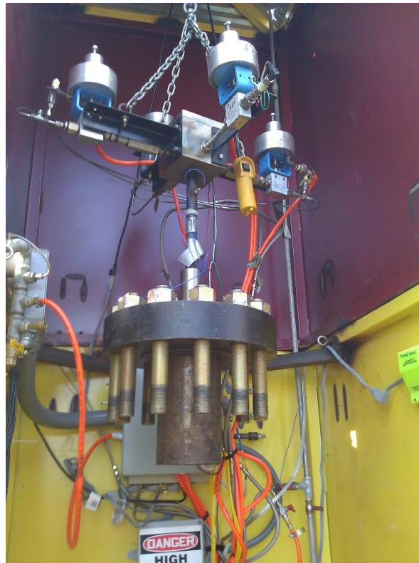
Figure 102: 20-L shock tube manifold suspended within bunker.
