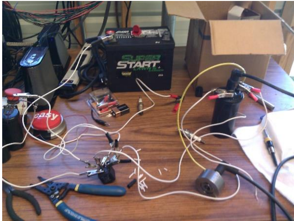
Figure 91: Buzz-coil/relay-driven spark ignition circuit.
