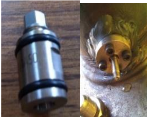
Figure 58: Isolating adapters used to minimize structure resonance noise.
