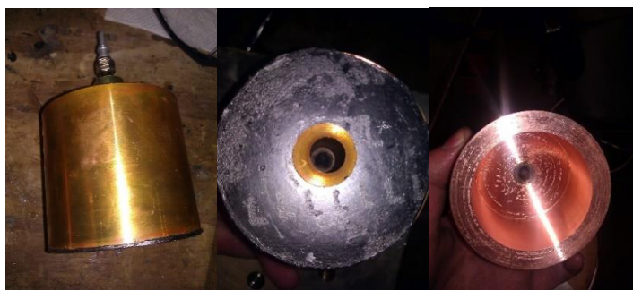
Figure 96: Glow plug adapter before and after boring out inner diameter.
