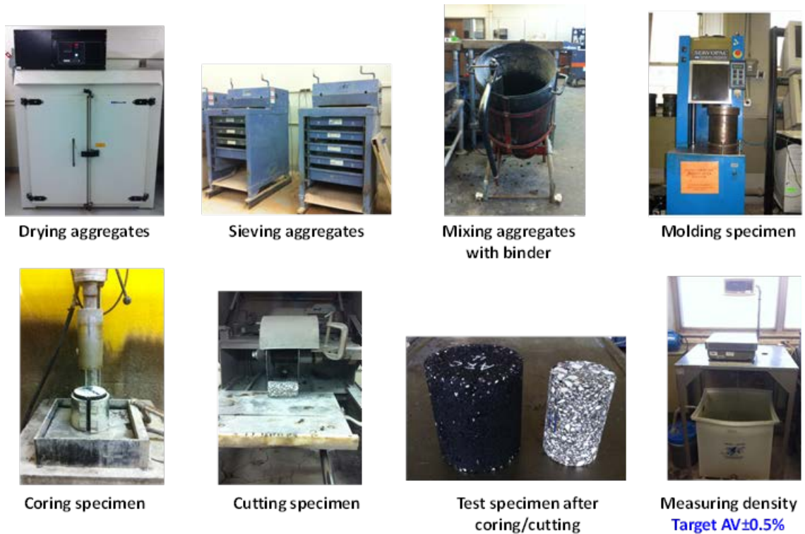
Figure 3.3 Steps for Preparation of Test Specimens
