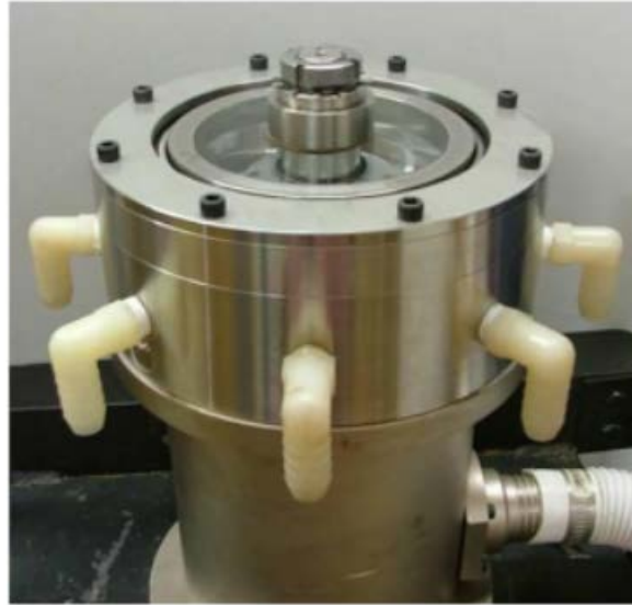
Figure 1-21: Two stage ESP setup (Barrios 2007)
