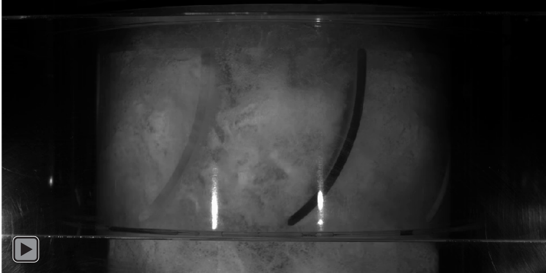
Figure 4-29: Video of the diffuser flow field at 1800 RPM, 50 psig inlet pressure, 12 kBPD liquid flow rate and 2% GVF
