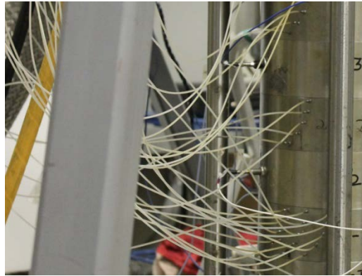
Figure 3-14: Static Pressure Taps on Diffuser
