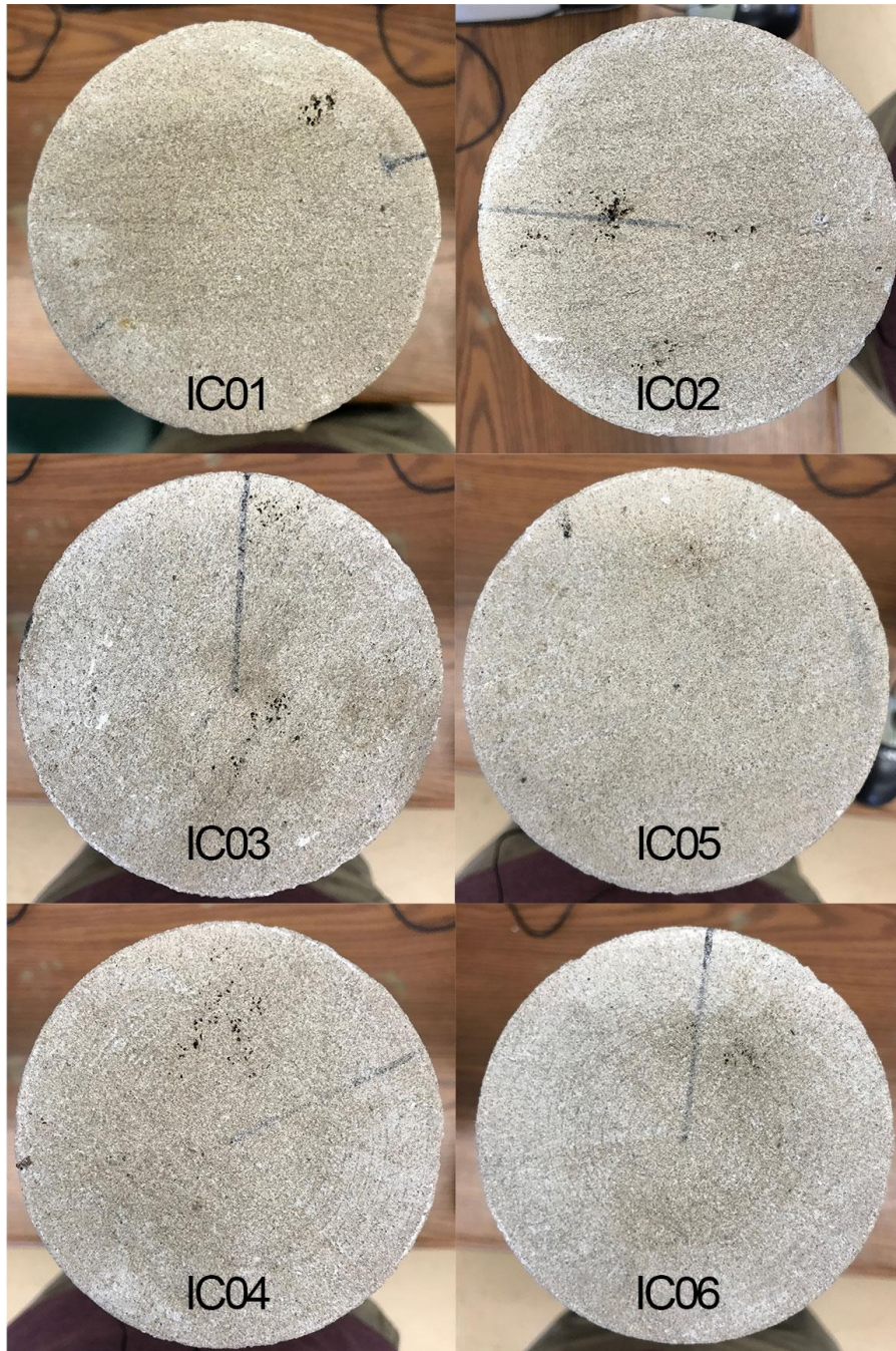
Figure A.2. Post-jetting core images showing wormholes (bottom view).
