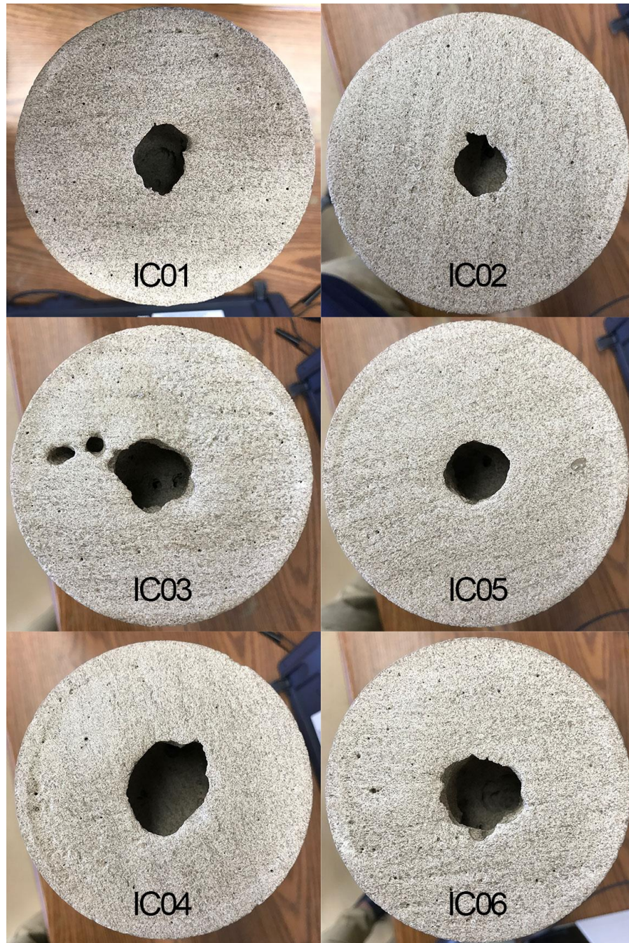
Figure A.1. Post-jetting core images showing cavities (top view).
