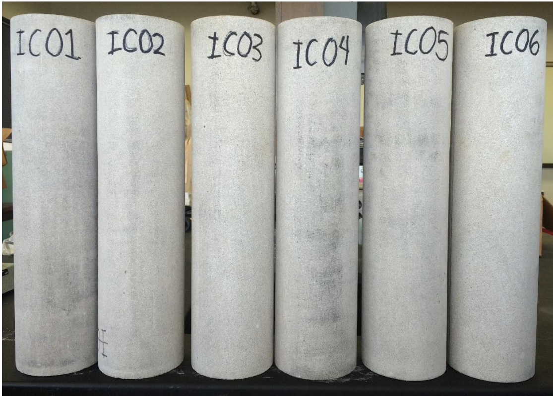
Figure 2.1. Indiana limestone rock samples used in the study.
