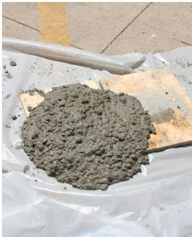
Figure 58. Significant Slump of Fresh Mix Without Steel Fibers
