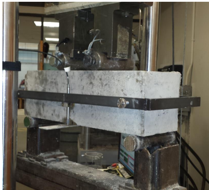
Figure 5. ASTM C1609 – Four Point Bending Test of Concrete Prism (6 in x 6 in x 20 in)
