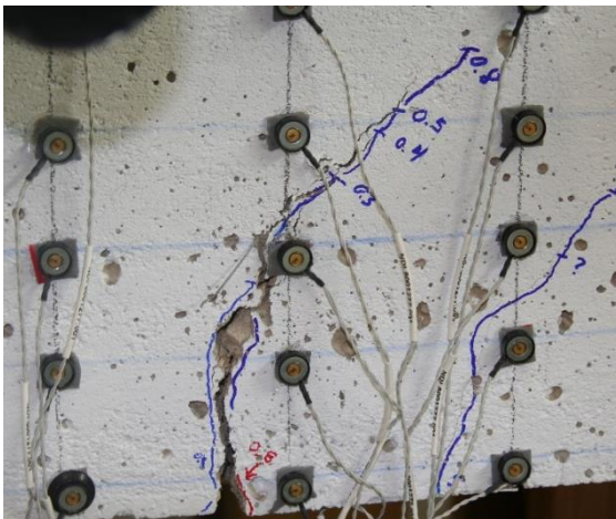
Figure 49. Crack Progression of W1 at Deflection Step: (a) 0.3 in deflection, (b) 0.6 in deflection, (c) 1.0 in deflection, and (d) 1.4 in deflection
