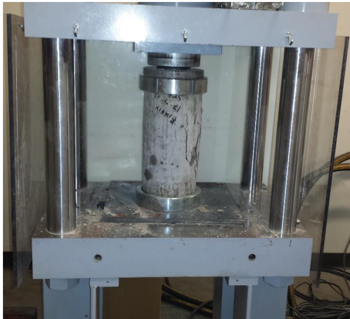
Figure 4. ASTM C39 - Compression of 6 in x 12 in Cylinder
