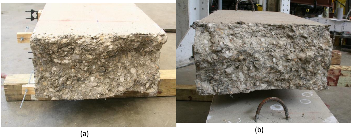
Figure 101. Fiber Distribution of S9020NOS00 (a) South Face of Failure Plane and (b) North Face of Failure Plane
