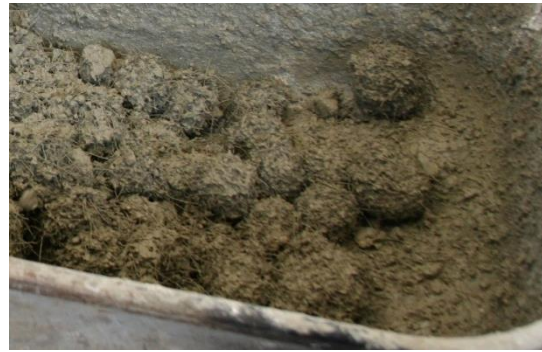
Figure 54. Significant Clumping in SFRC
