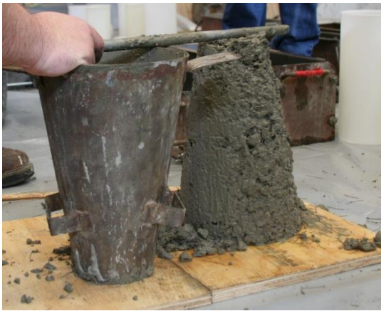
Figure 53. 2.0% SFRC Lack of Slump
