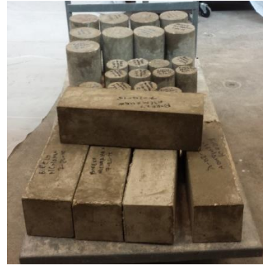
Figure 61. Casts for ASTM Materials Tests on Way to Curing Room
