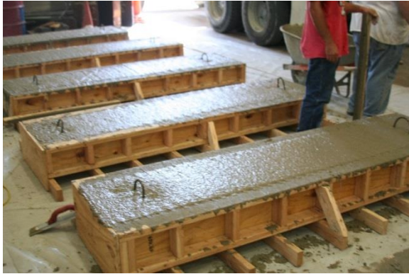
Figure 60. Five of Twelve Completed SFRC Slab strips
