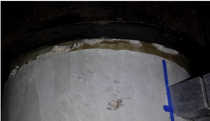
Figure 66. Failure of SFRC Cylinder in Epoxy-Concrete Interface ( V_f = 0.5\% , Sample 1)
