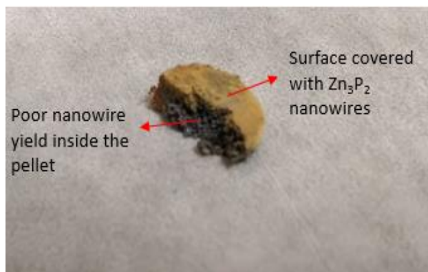
Figure 13: Photograph of the pellet with nanowires only on the surface of the pellet. The inner region of the pellet was found to have some unreacted zinc material along with Zn_3P_2 nanowires
