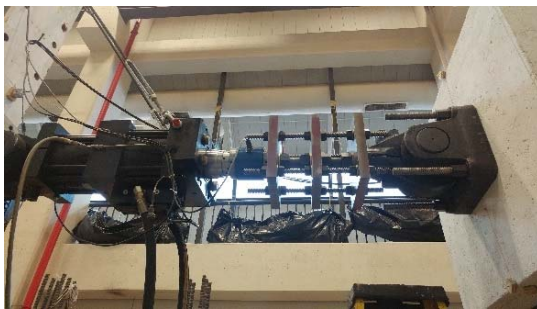
(c) Installed HT Actuator
