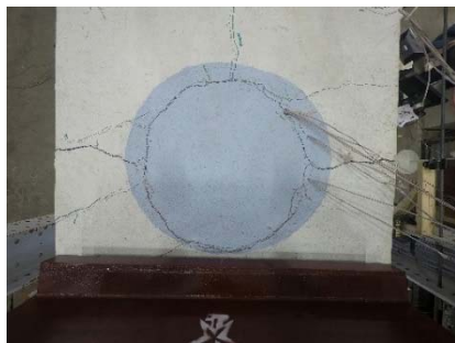
Figure 4.3. Visual Observations at Failure; Blue paint extends beyond edge of pocket in RCS-16-12. (Left: RCS-16-12, Right: PSS-16-12)
