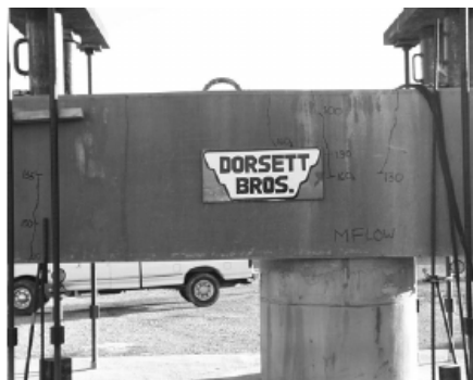
(a) Flexure Cracks on Sidewall at Factored Loads
