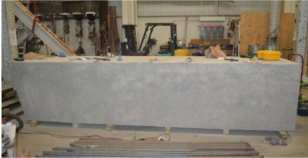
(a) Honeycombing Repairs – Front Face of Bent Cap
