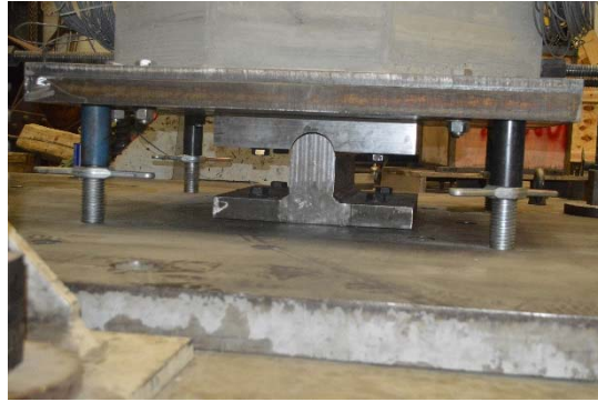
Figure 3.65. Installed Roller Foundation Assembly onto Test Setup.
