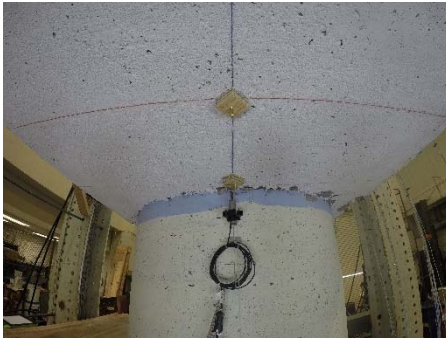
Figure 4.14. Crushing at Interior Face of Column – RCS-16-12.
