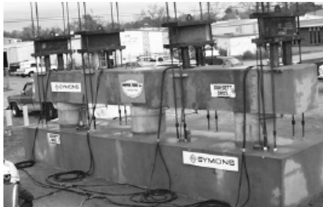
Figure 2.11. Experimental Setup Column Bent Cap (Matsumoto et al., 2001).
