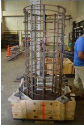
(b) Deformed Spiral
