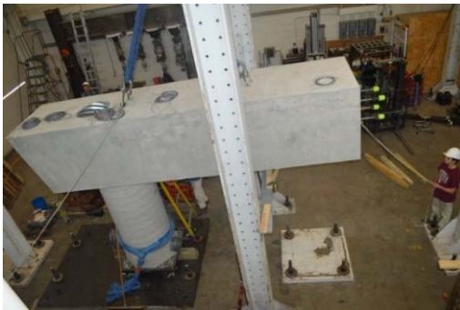
(c) Placed Bent Cap Top View
