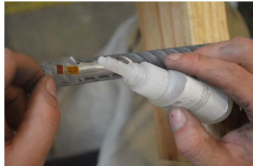
(f) Application of M-Bond 200 Adhesive
