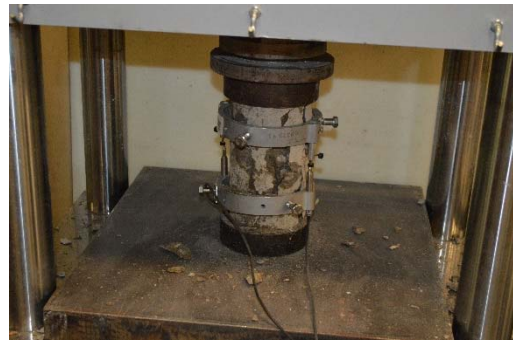
(b) Modulus of Elasticity
