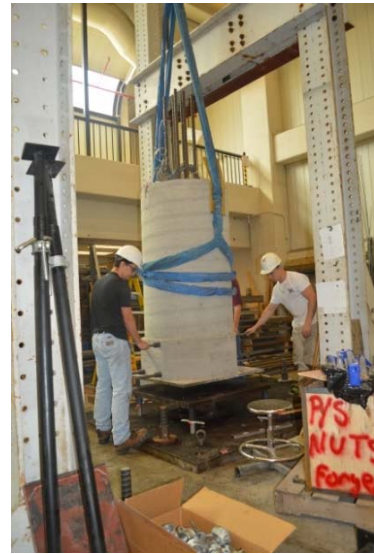
(b) Installing onto Test Setup
