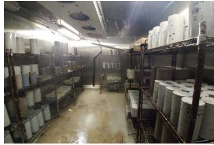
(b) Curing Room
