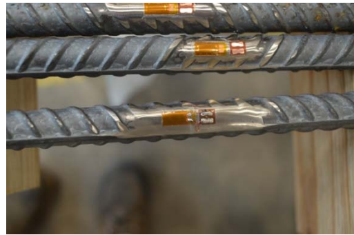
(b) Soldered Ports
