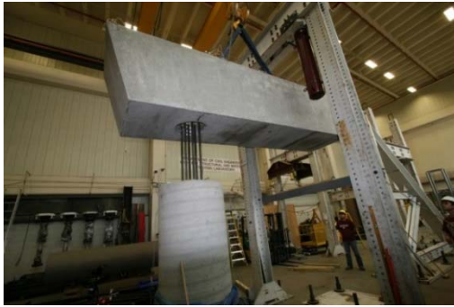
(a) Placing Bent Cap
