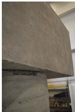
Figure 3.54. Honeycombing in Bedding Layer – Front Face.
