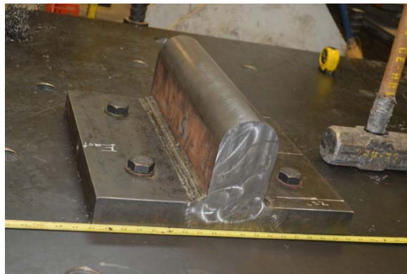
Figure 3.62. Installation of Roller onto 10-ft x 7-ft Base Plate.
