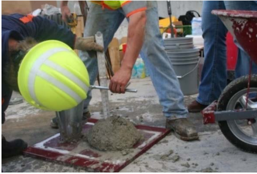
(a) Slump Test
