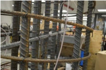
Figure 3.42. Temporary Dowel Formwork.
