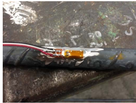
(b) Application of M-Coat A
