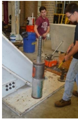
Figure 3.56. Post-tensioned Dywidag Connection to Strong Floor.
