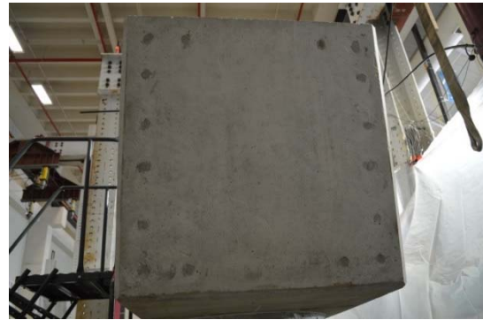
(b) Grout Strand Patches
