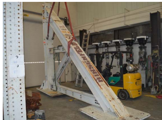
(b) Top Horizontal Reaction Frame
