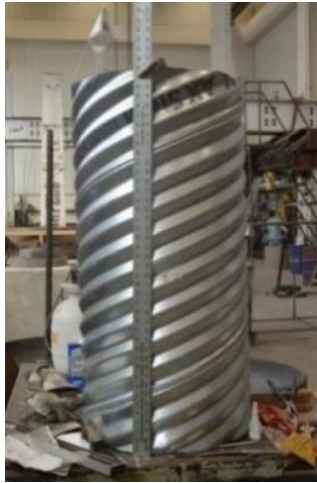
Figure 3.11. 21-in Nominal Diameter, 12-gage Steel Corrugated Pipe.
