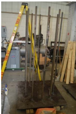
(a) Threaded Longitudinal Bars
