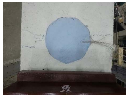
Figure 4.3. Visual Observations at Failure; Blue paint extends beyond edge of pocket in RCS-16-12. (Left: RCS-16-12, Right: PSS-16-12)
