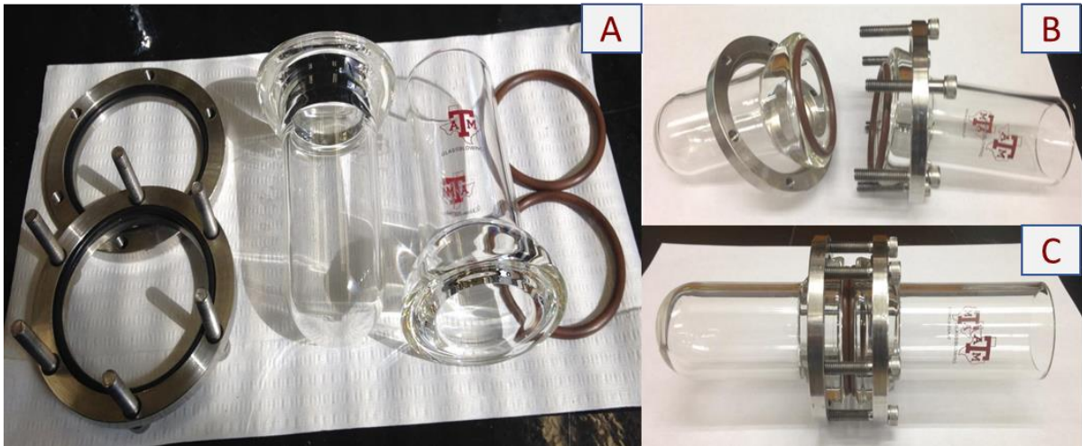
Figure 10: Digital photographs of the filtration parts and how they are assembled for deployment under high-pressure and high-temperature conditions.
