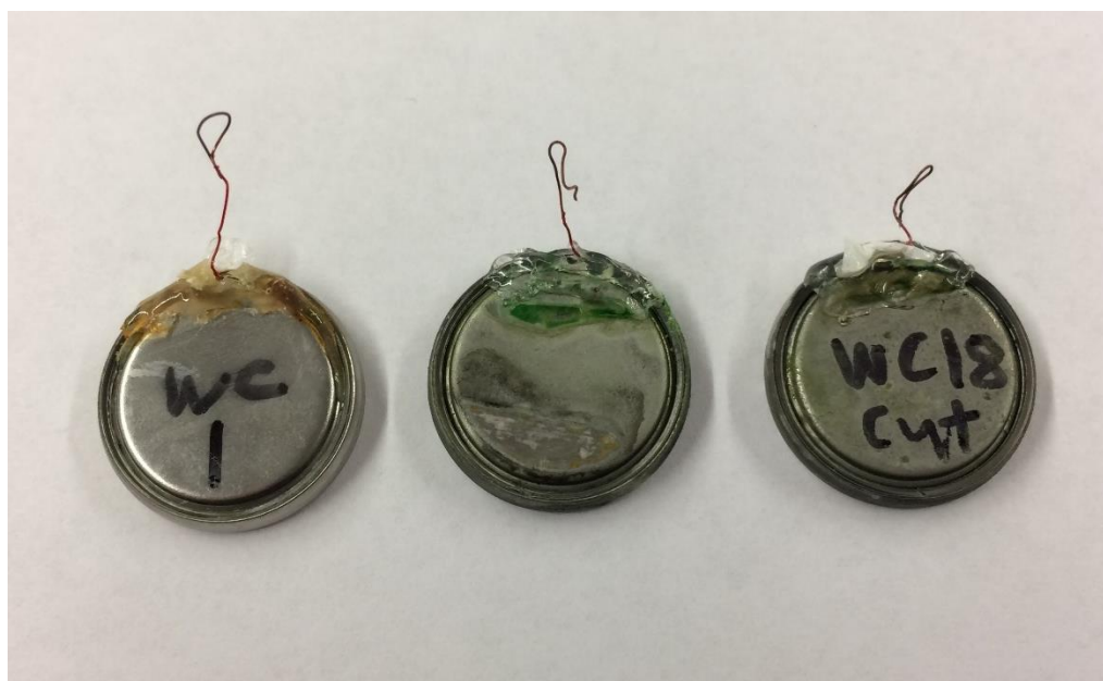
Figure 20 Improperly sealed three-electrode coin cells, demonstrating leaking and resultant reaction of the electrolyte with the environment.
