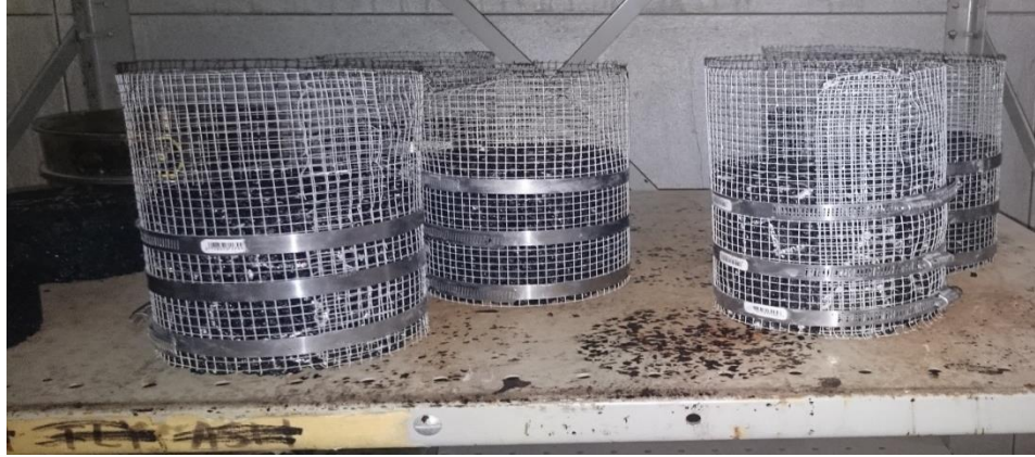
Figure 25. Brace for preventing collapse of the mixture in some conditioning protocols.
