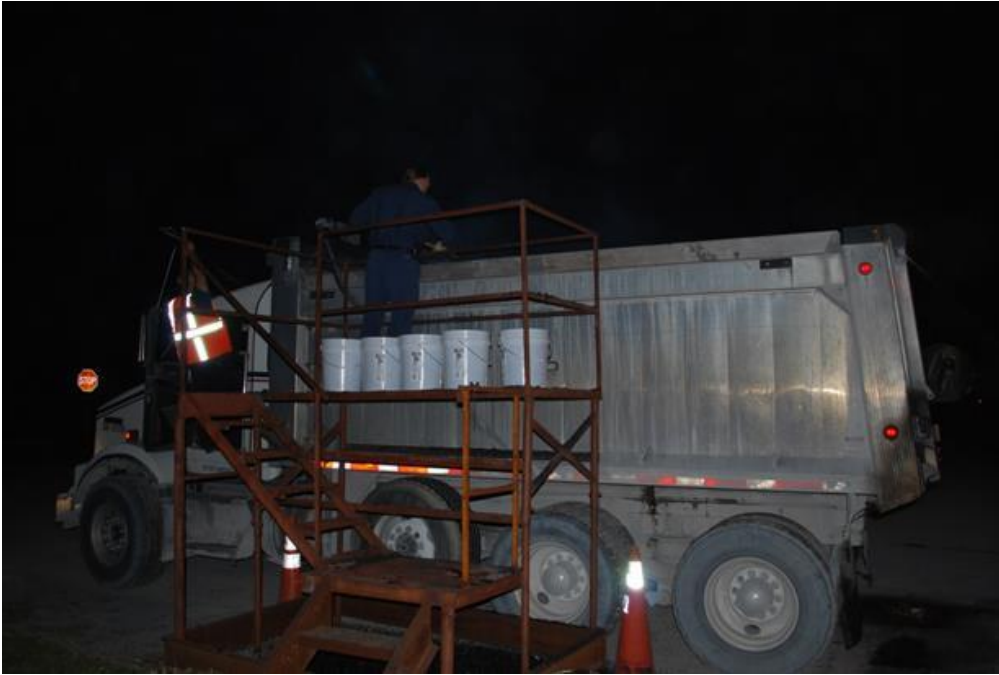
Figure D5. Plant mixture sampling from dump truck at the plant.
