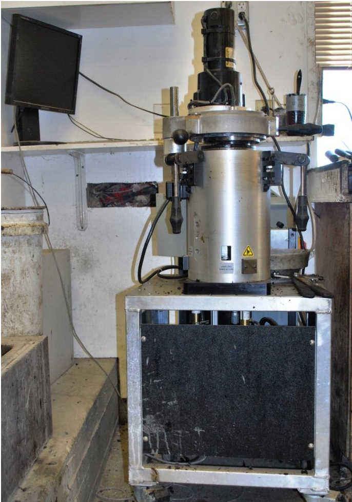
Figure E6. Pine Brovold Superpave Gyrotory Compactor used in the Plant Lab.
