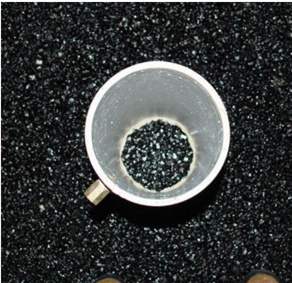
Figure D8. Inside view of the WFV test cylinder after application of the sealing putty.
