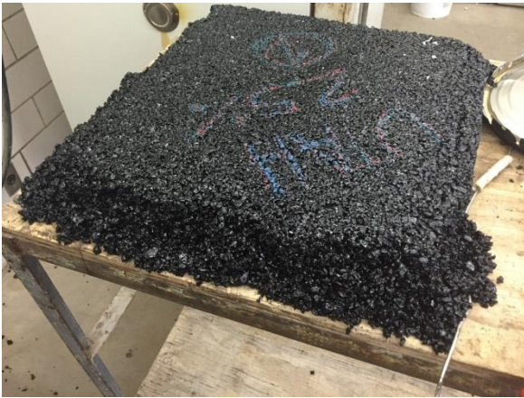
Figure 29. Slab compacted with material from Utah.
