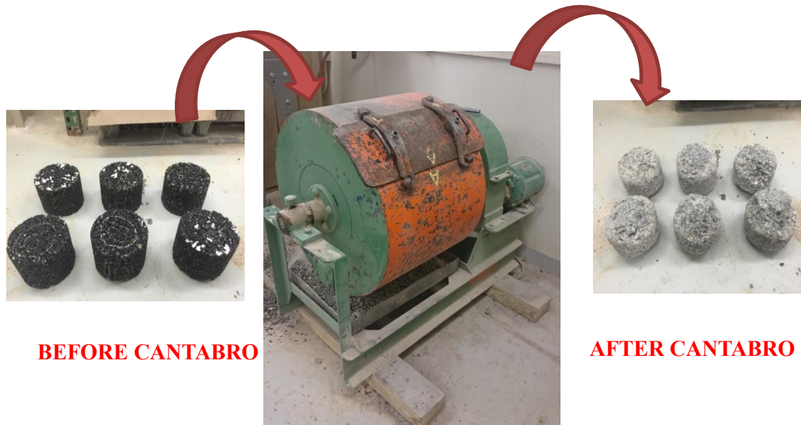
Figure 22. Los Angeles abrasion machine, Cantabro loss test setup.
