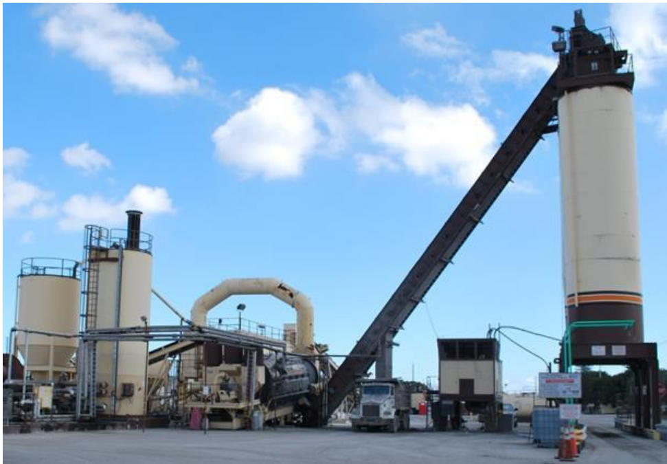
Figure D3. Pompano Beach drum plant where the OGFC mixture was produced.
