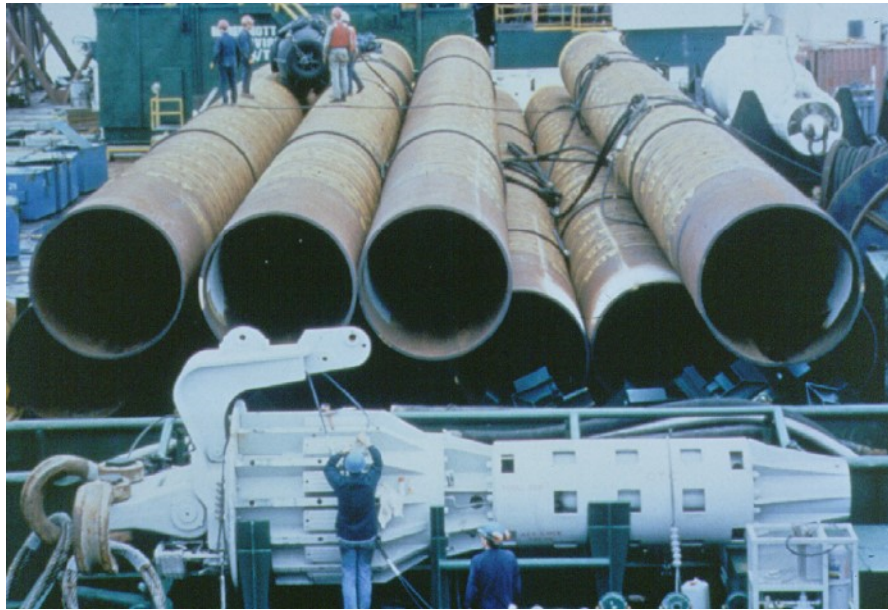
Figure 1.3: Offshore piles with installation hammer (white). (Courtesy of Dr. James D. Murff)
