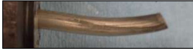
Figure 4-12: U-10Zr rod from extrusion 3
