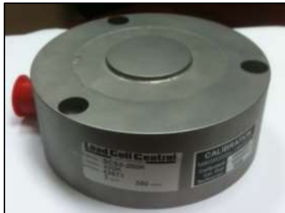
Figure 3-3: The load cell used for all extrusion experiments
