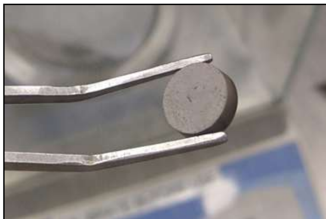
Figure 3-32: U HDH pellet representative of all low density pellets created
