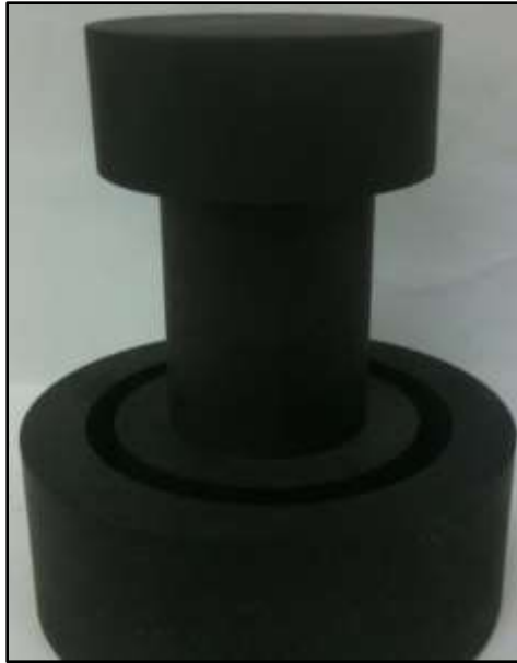
Figure 3-29: Graphite casting mold assembled
