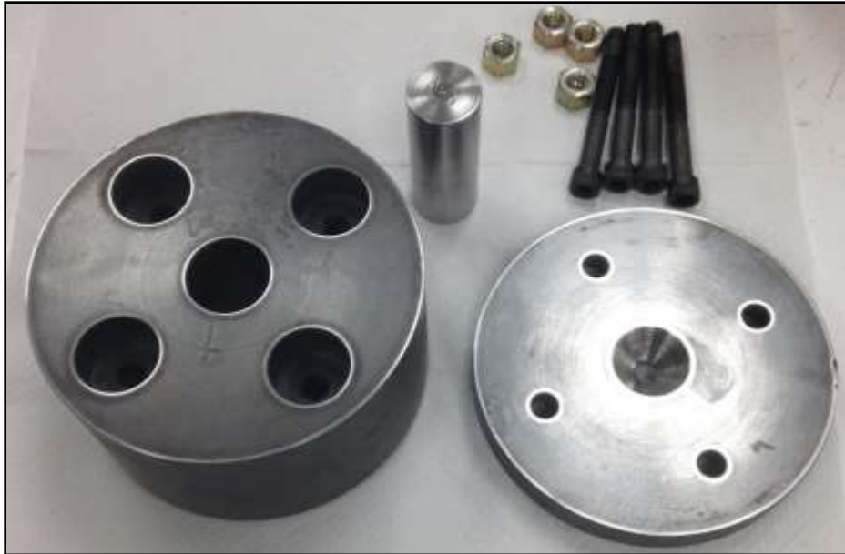
Figure 4-13: Extrusion tooling before use in extrusion 4
