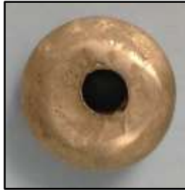
Figure 4-46: U billet used in extrusion 9
