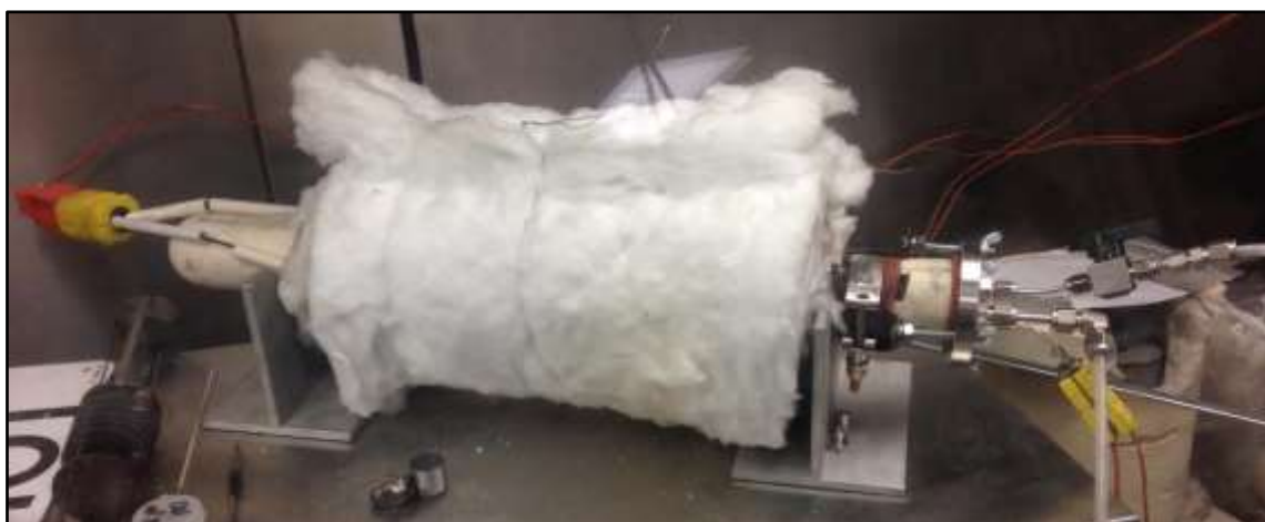
Figure 3-30: Hydride/de-hydride system located inside of an inert atmosphere glovebox.
