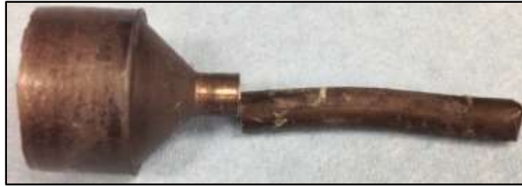
Figure 4-5: U-10Zr rod from extrusion 2
