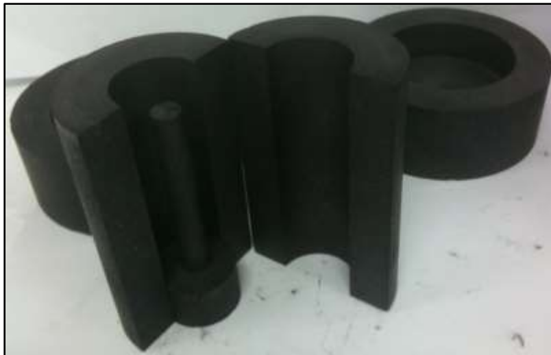
Figure 3-28: Graphite casting mold disassembled
