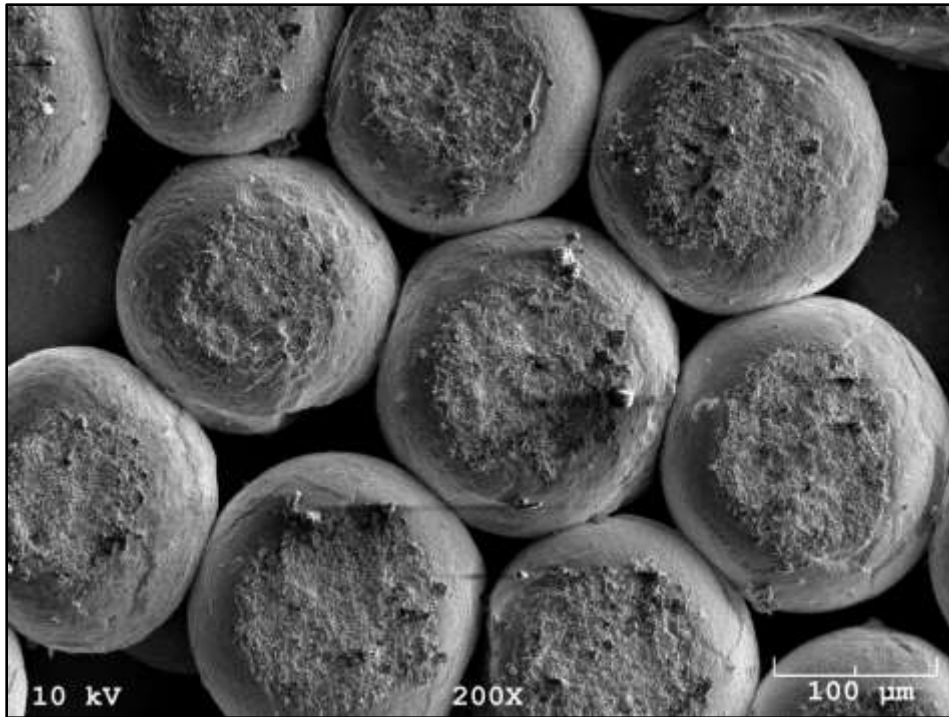
Figure A5-49: 80.96% TD U-10Zr spheres pellet (26-120) at 200X (surface)
