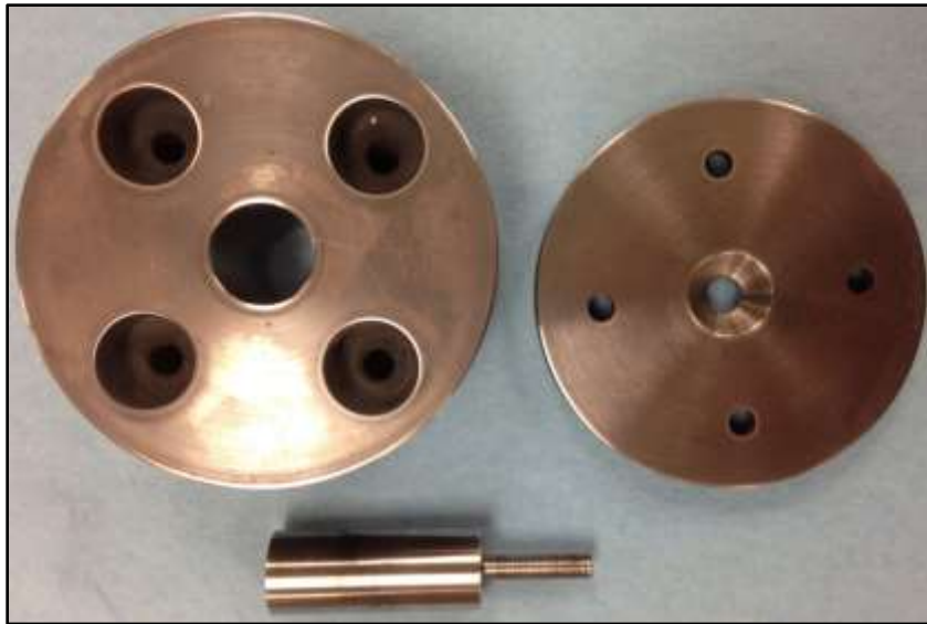
Figure 4-38: Extrusion 7 tooling before use
