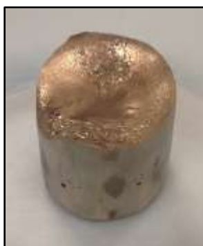
Figure 4-33: U-10Zr billet for extrusion 13
