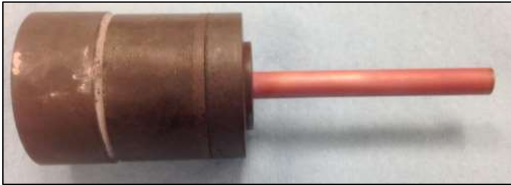
Figure 3-20: Copper tube from tube extrusion test 3
