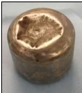
Figure 4-55: Uranium billet for extrusion 12
