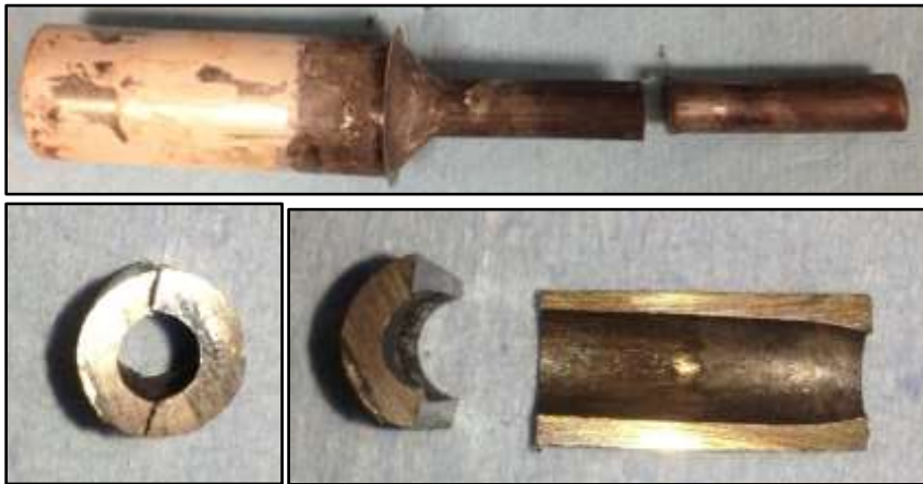
Figure 4-39: Multiple pictures of the U tube from extrusion 7
