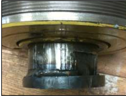
Figure 3-2: Press head before repair
