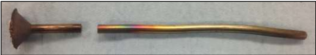
Figure 4-56: U rod from extrusion 12 after a small section was removed
