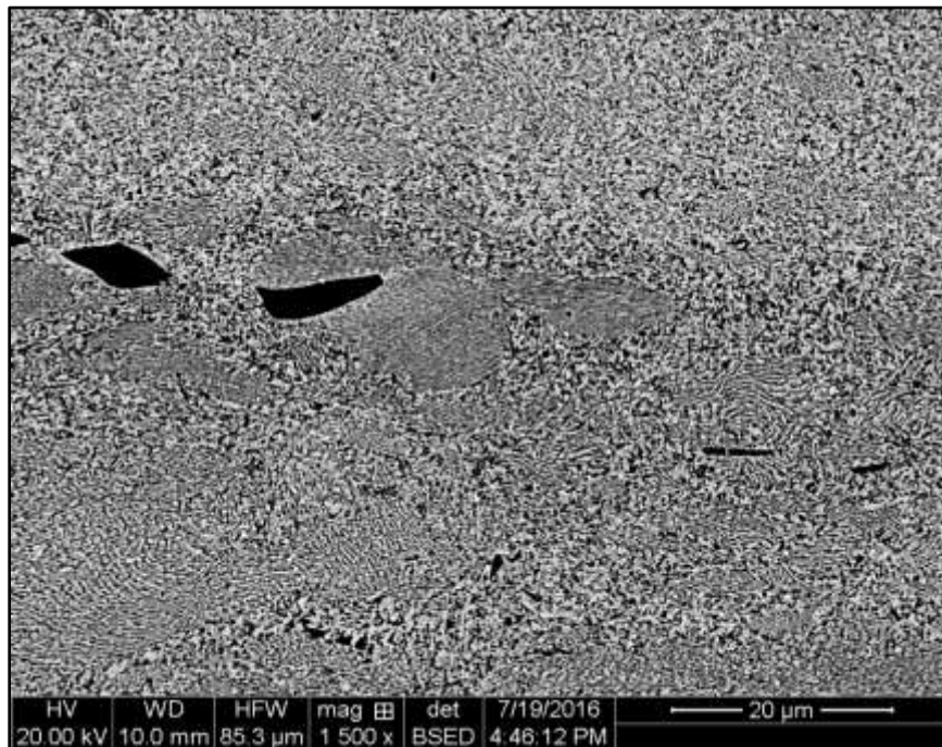
Figure A7-13: BSE image of extrusion 11 U-10Zr rod
