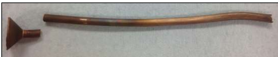
Figure 4-34: U-10Zr rod from extrusion 13
