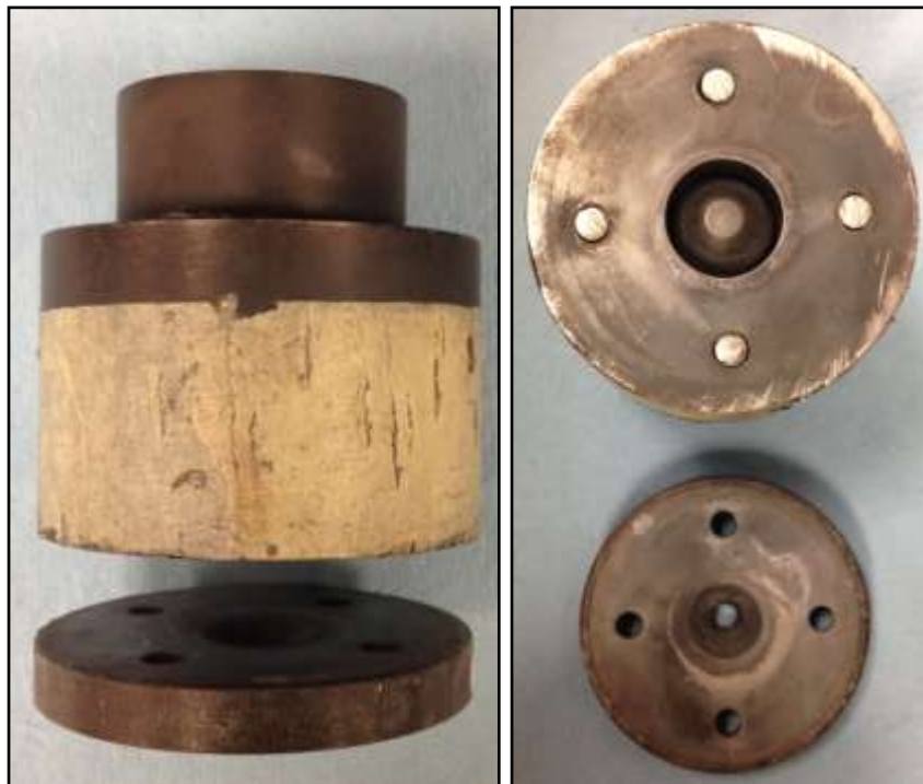
Figure 4-7: Multiple views of tooling used in extrusion 2
