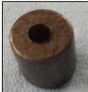
Figure 3-27: Uranium billet with central hole
