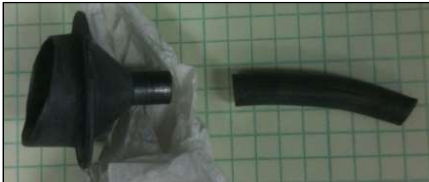
Figure 4-4: U-10Zr rod from extrusion 1
