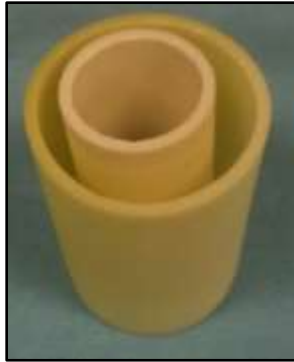
Figure 3-24: Primary Y 2 O 3 crucible in a secondary Y 2 O 3 crucible
