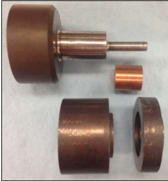
Figure 3-19: Extrusion tooling used in copper tube test 3
