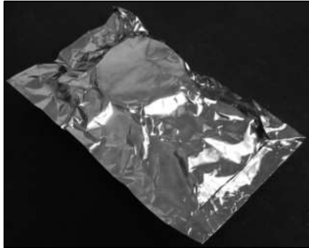
Figure 3-7: Extrusion tooling sealed in steel foil
