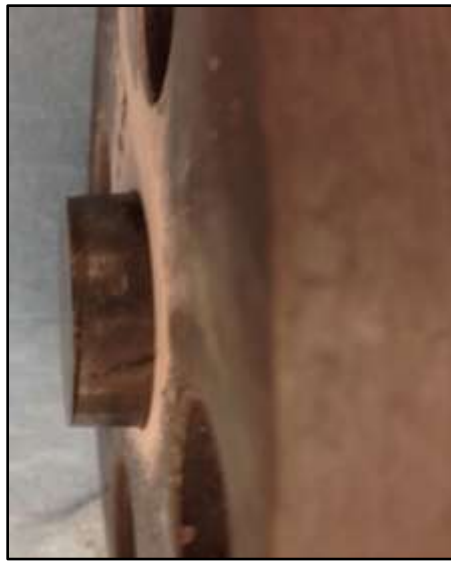
Figure 4-24: Failed ram of extrusion 6
