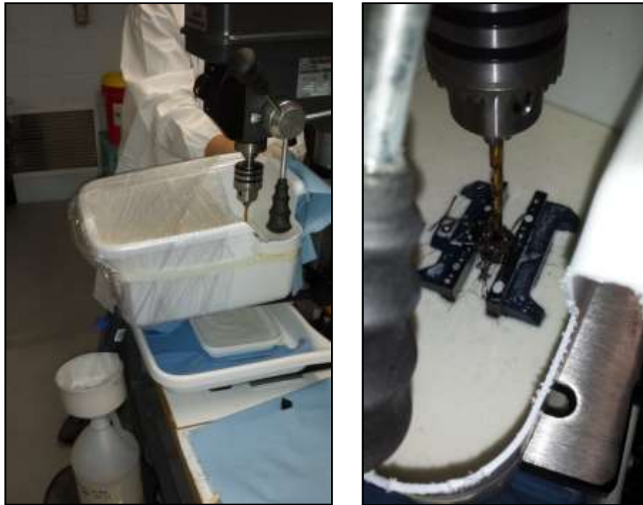
Figure 3-26: Drilling equipment for uranium billets
