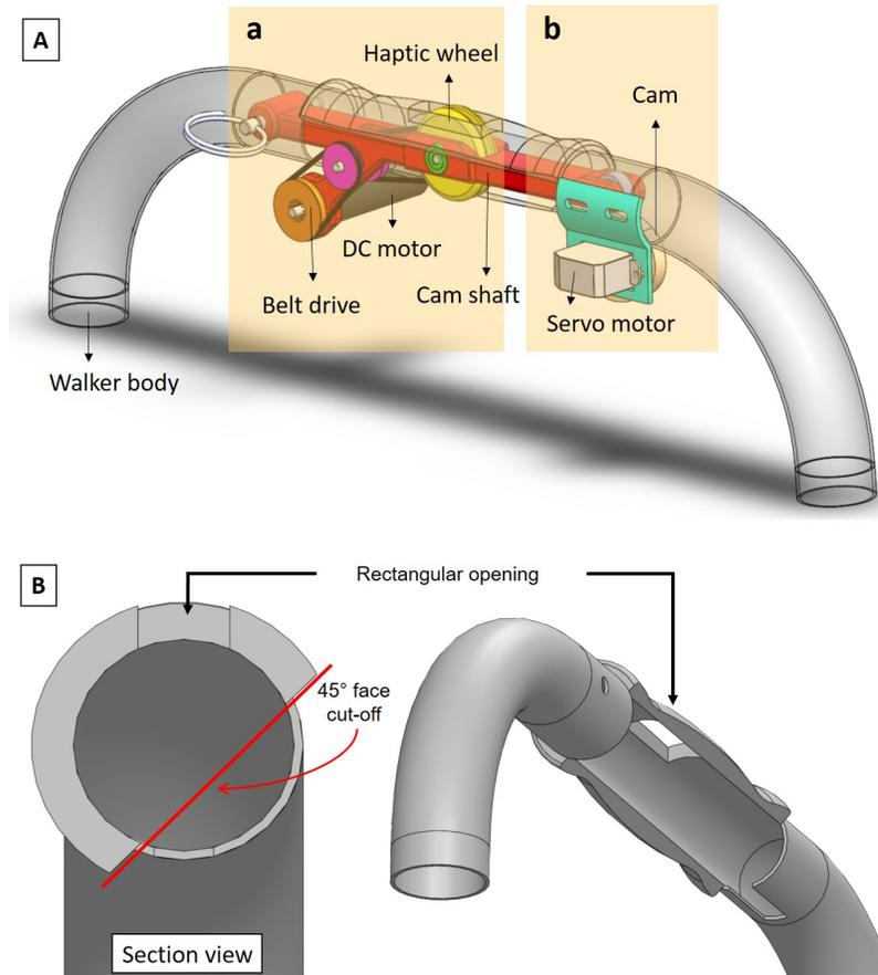
Figure 6.3: (A) CAD design of the skin stretch device embedded into the right-hand side handgrip of a walker. The mechanism consists of two parts for producing lateral skin stretch using a DC motor (a) and normal skin displacement using a micro servo (b). (B) Section view and bottom front view of handgrip tube. Two sites including a rectangular opening on the top and a 45° face cut-off along the tube were fabricated for the installation of the skin stretch device.
