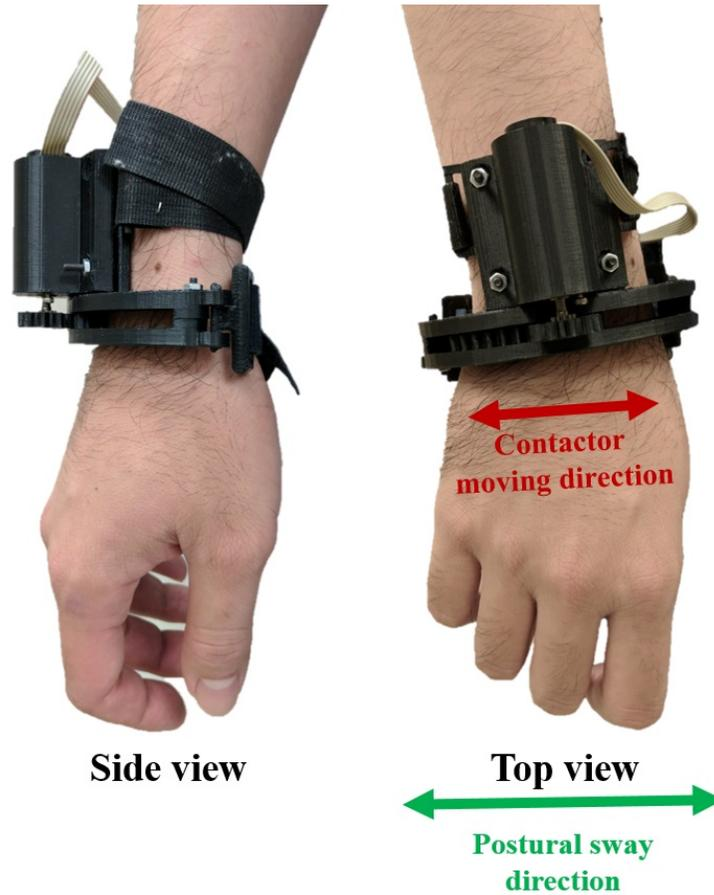
Figure 5.3: Skin stretch device worn by subject viewed from the side and the top. The contactor moves along the top of wrist surface in response to the subject's postural sway direction.
