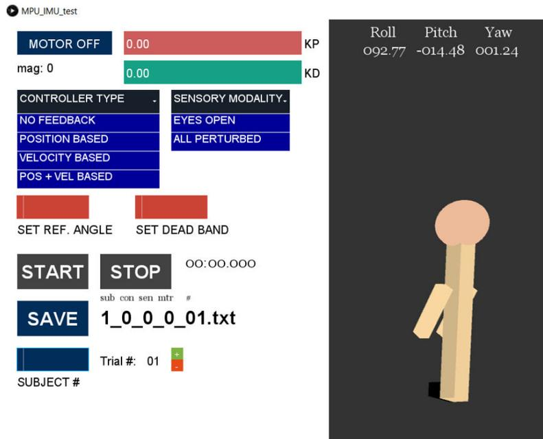
Figure 6.10: Graphical user interface for real-time posture visualization, user I/O and data acquisition.
