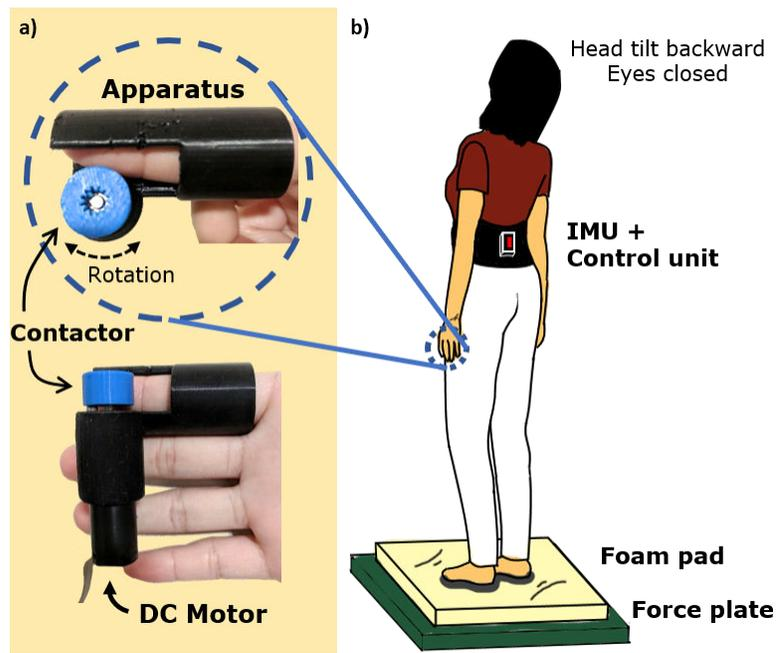
Figure 4.1: Sensory augmentation system and experiment setup. a) The sensory augmentation device induces skin stretch at an index fingertip pad with a rotating contactor. The rotating motion of the contactor is controlled by a DC motor. b) In the experiment, subjects were asked to tilt their head up with eyes closed, while standing on a foam pad on the force plate.
