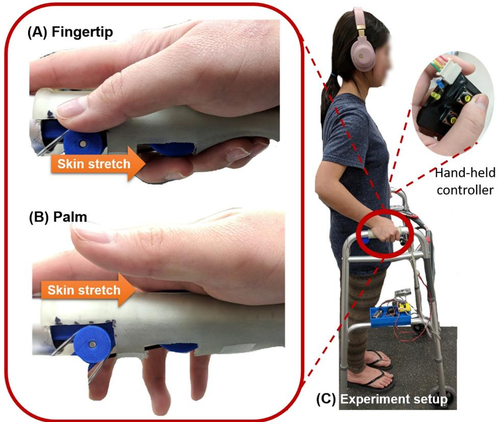
Figure 6.5: Experiment setup. During the experiment, skin stretches are applied at different locations in the fingertip session (A) and palm session (B). (C) The participant stands quietly while holding the handgrip using her right hand and a controller using the left hand to toggle between two directions.
