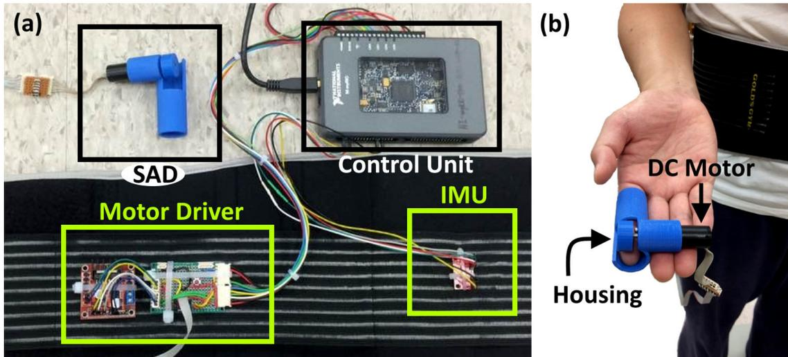
Figure 3.2: System overview. (a) The system consists of a sensory augmentation device (SAD) that induces the skin stretch at an index fingertip pad. A control unit, motor driver, and IMU are enclosed in a waist belt. (b) DC motor is mounted at the housing of SAD where subject’s index finger is inserted. Cutaneous skin stretch feedback is therefore provided by the shearing between contactor operated by the DC motor and fingertip pad.
