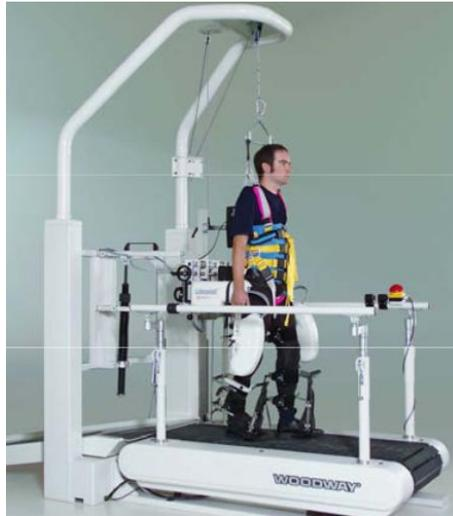
Figure 2.3: Lokomat gait orthosis for lower-limb balance and gait training. Reprinted from [2].
