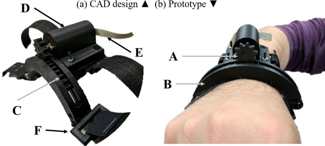
Figure 5.2: Wrist-worn skin stretch device. Skin stretch feedback is provided by the contactor connected to a curved rack (C). The rack is driven by a DC motor (E) with a custom pinion (A) attached (D: motor housing). The rack and pinion mechanism is housed inside two combined curved bands with the embedded track (B). Two movable buckles (F) are attached at each end of bands to accommodate various wrist sizes. User can wear and tighten it using two adjustable Velcro straps.
