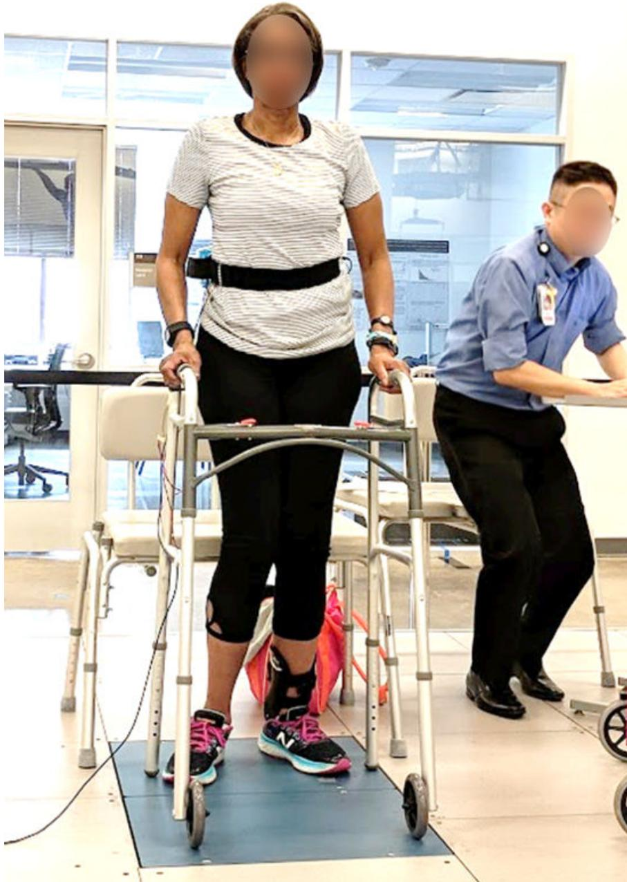
Figure 6.11: Experimental setup for the MS subject in performing static balancing tasks with the sensory augmentation walker. Subjects were spotted by a physical therapist (right) to ensure safety during the experiment.
