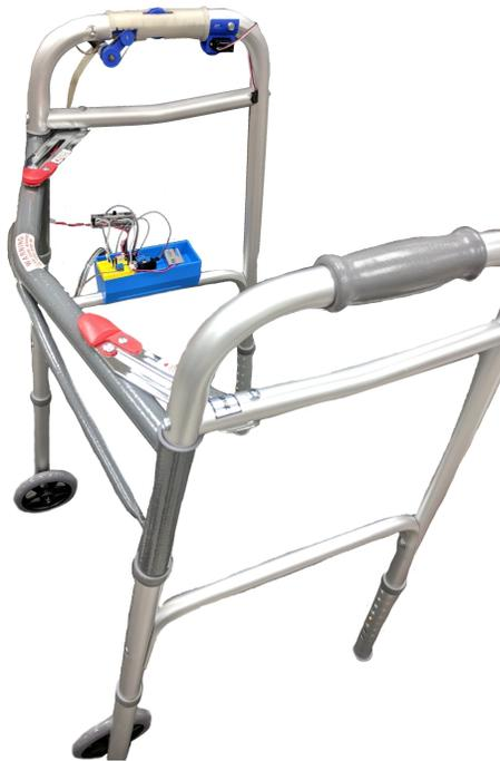
Figure 6.1: A standard front-wheel walker with the sensory augmentation system that includes: (i) a skin stretch feedback device embedded into the right handgrip and (ii) a control unit together with the power source packed at the lower part of the walker.
