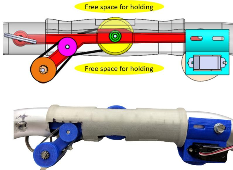
Figure 6.4: CAD design (top) and the prototype (bottom) of the skin stretch device from the left-side view.
