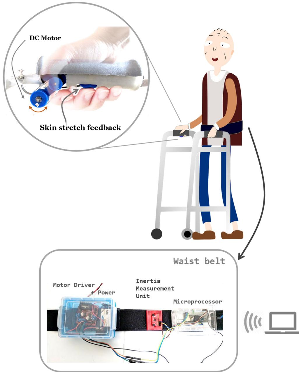
Figure 6.9: System overview of the sensory augmentation walker. The entire system consists of a waist belt that encloses the IMU, microprocessor, motor driver and power source and a conventional four-wheeled walker that integrates a skin stretch feedback device at the grip. Data is transmitted through a USB cable for real-time data logging and data collection.
