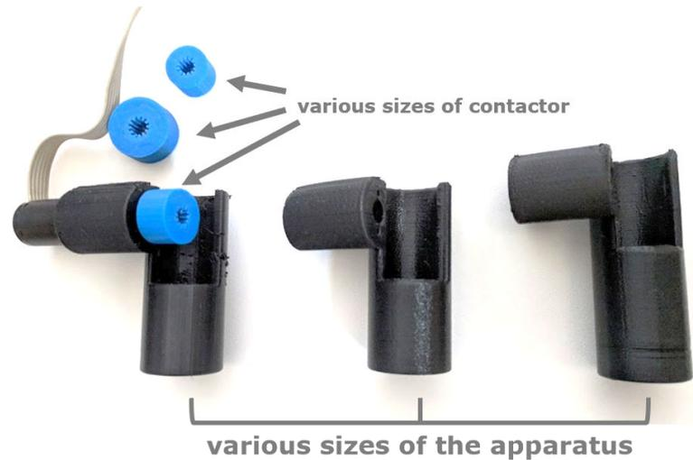
Figure 4.2: Various sizes of the feedback apparatus and contactors.
