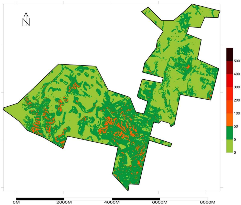
Figure 4-7 RUSLE predicted soil erosion (tons/acre/year) for Bastrop State Park
