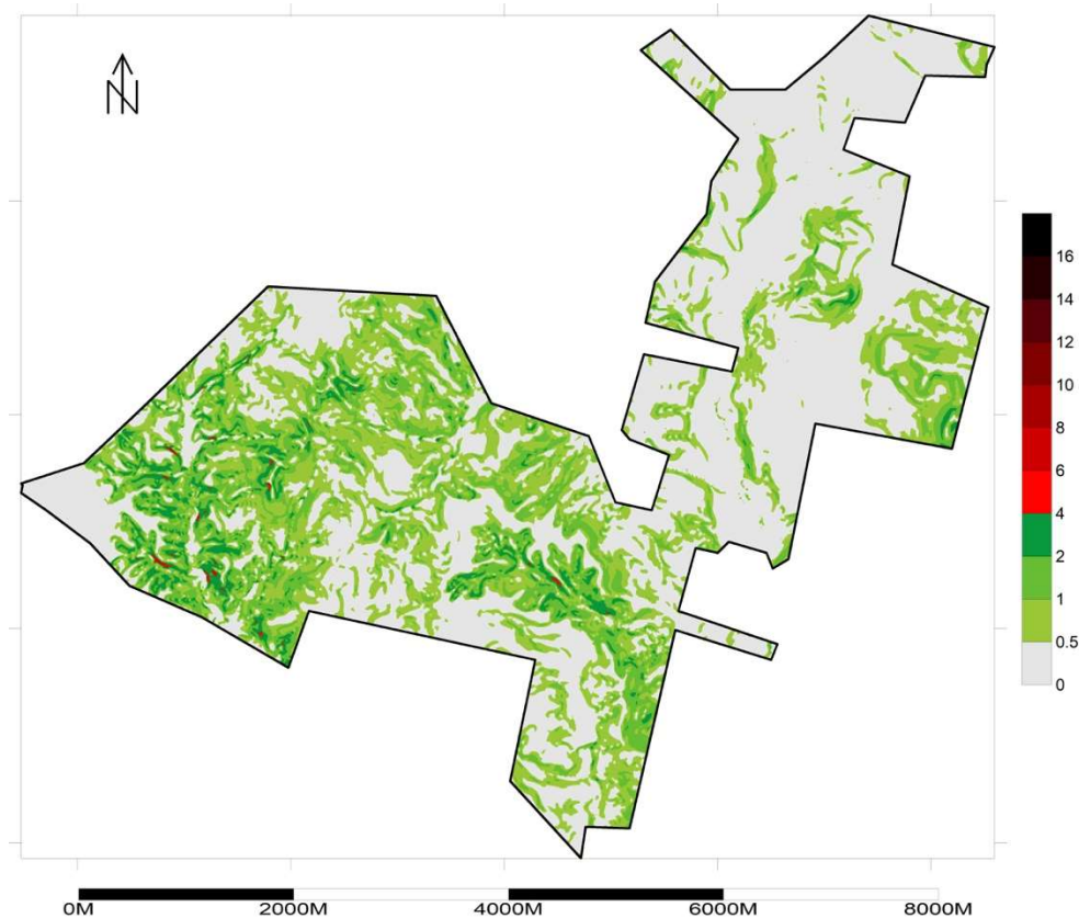
Figure 4-4 Bastrop State Park Slope Length and Steepness LS- Factor
