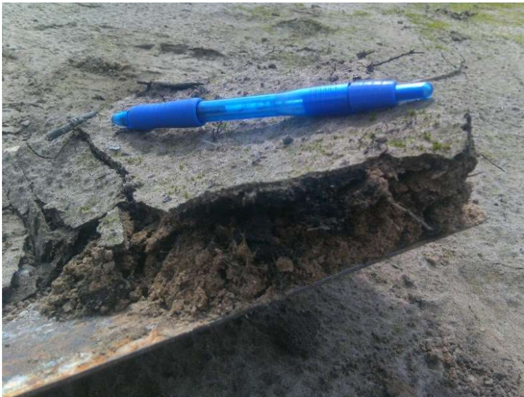
Figure 3-6 An ash crust developed in the heavily burned areas of the study site after moisture re-entered the environment.
