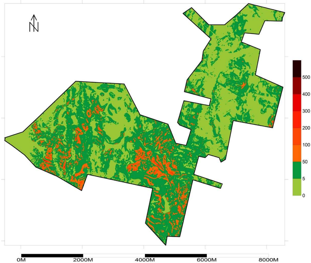
Figure 4-8 RUSLE predicted soil erosion (tons/acre/year) for Bastrop State Park with water repellent soils
