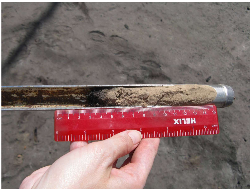
Figure 3-2 Soil Sampler and handheld ruler used to measure ash depth
