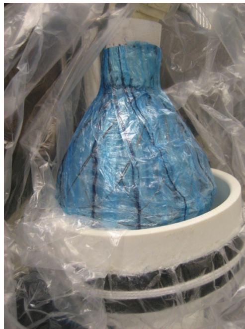
Figure 28. Cardiac support device (top) Prototype of the model which is used to measure EDPVR of a normal heart (bottom) Prototype of the cardiac support device on the heart model.
