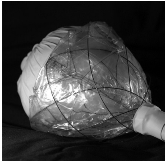
Figure 9. A prototype of the polymeric multi-chambered support device deployed about an excised ovine heart that is preserved and wrapped in thin latex for handling.
