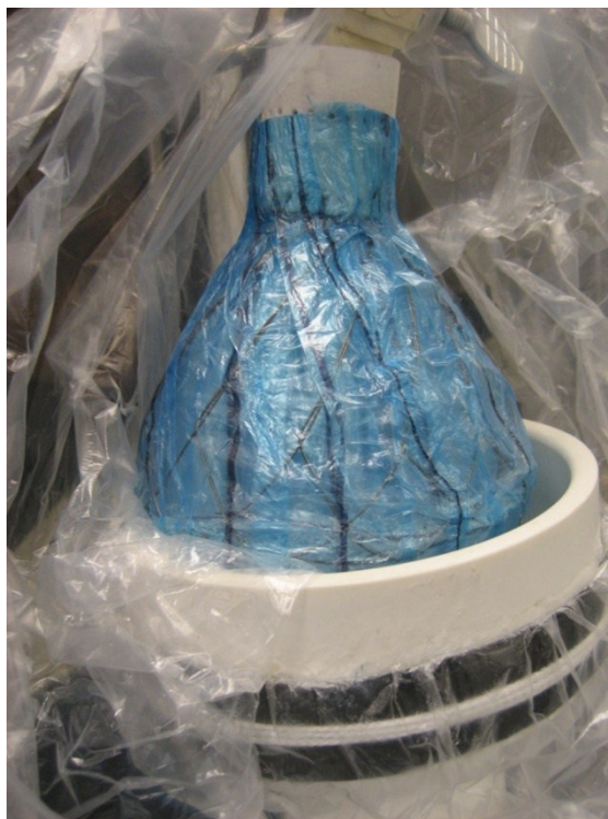
Figure 17. Cardiac support device (top) Schematic design of the inflated cardiac support device placed on the heart model in the experimental setup; (bottom) Prototype of the cardiac support device on the heart model which is used measure EDPVR.
