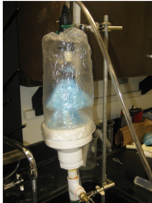
Figure 30. Diastolic recoil device (top) Schematic design of the inflated diastolic recoil device placed on the heart model in the experimental setup; (bottom) Prototype of the diastolic recoil device inside the pseudo pericardial sac.
