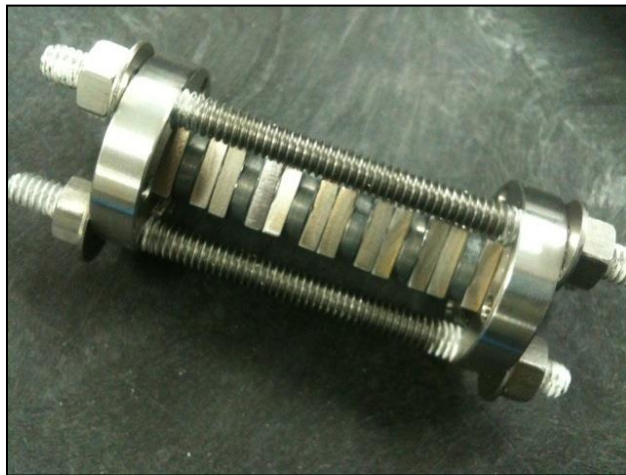
Figure 3-3. Assembled diffusion couple stack in jig.
