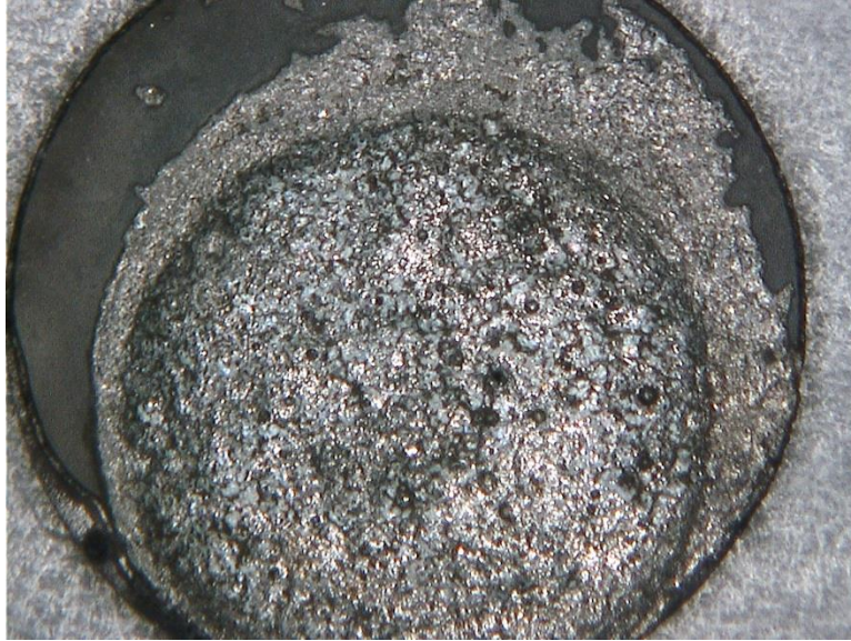
Figure 4-21. Remaining iron disk following exposure to Nd for 28 days at 550°C.
