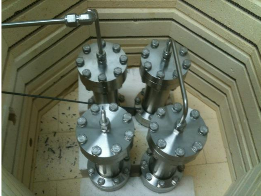
Figure 3-4. Diffusion couples loaded into kiln prior to heat treatment.
