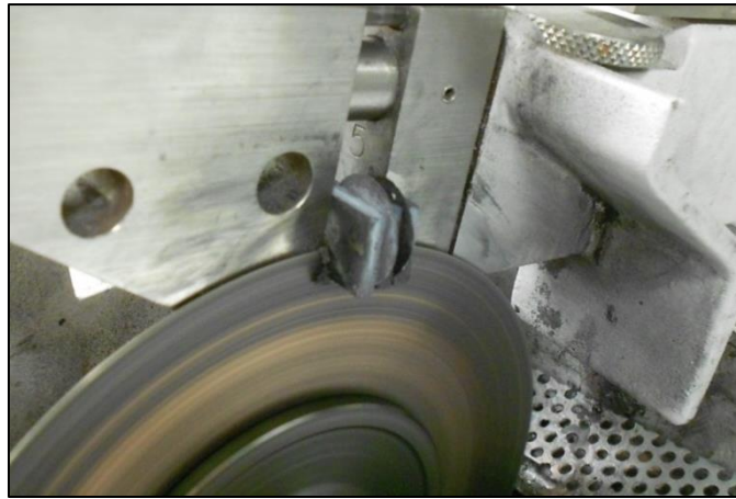
Figure 3-5. Diffusion couple sectioning using diamond saw.
