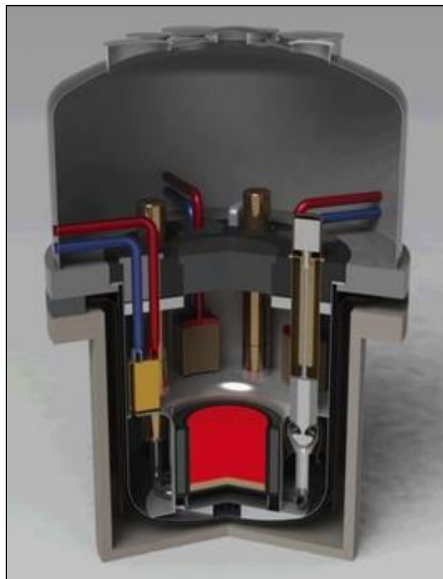
Figure 2-1. Cutaway diagram of conceptual TWR design [12].
