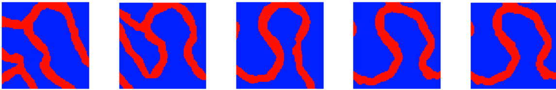
Fig. 3.14 – The best facies model (solution) after 100 (1st column), 500 (2nd column), 1000 (3rd column), 5000 (4th column), and 10000 (last column) iterations for Example 3.3 where adaptive facies conditioning from multiple TIs is used.
