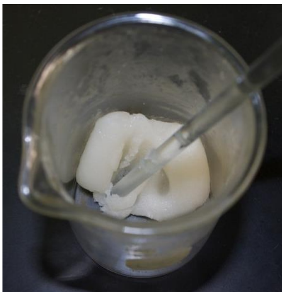
Figure 11 Image of a laboratory-scale, hand-mixed AP-HTPB propellant.
