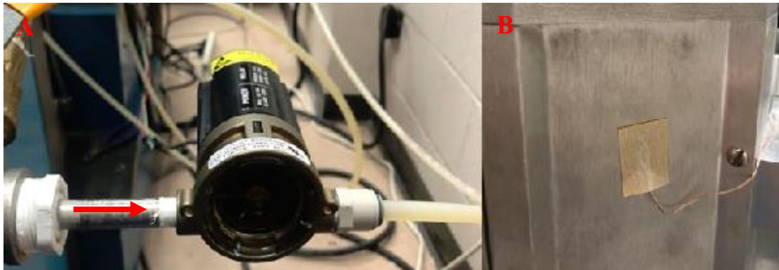
Figure 11. A) Flow switch B) thermostat switch
