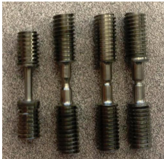
Figure 12. Machined samples with notches according to Bridgman's equation
