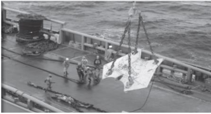
(e) Vertically-loaded anchor (courtesy of C. Aubeny).
