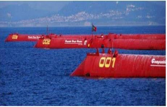
(c) Pelamis wave energy converter (courtesy of Sounds & Sea Technology).
