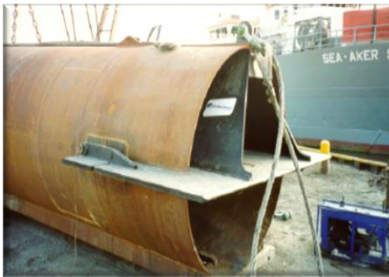
(f) Suction-embedded plate anchor (courtesy R Wilde, Intermoor).
