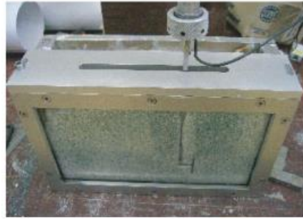
Figure 2.33 Geometrical notation and testing chamber with installed plate Anchor (after O'Loughlin et al. 2006).
