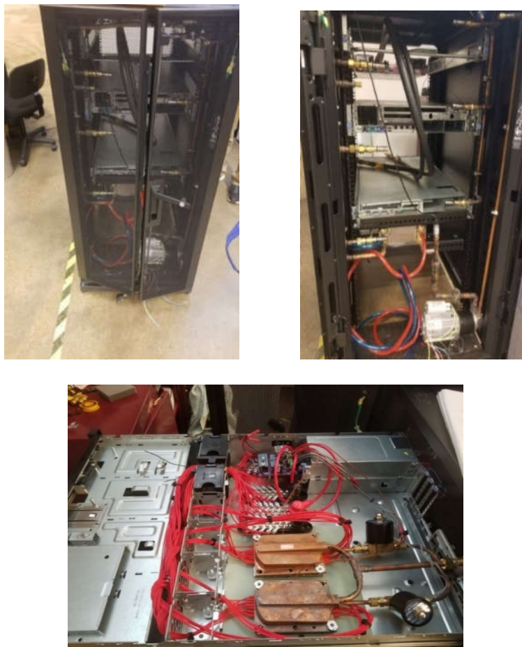
Figure 12: Prototype PTP cooling system for server banks
