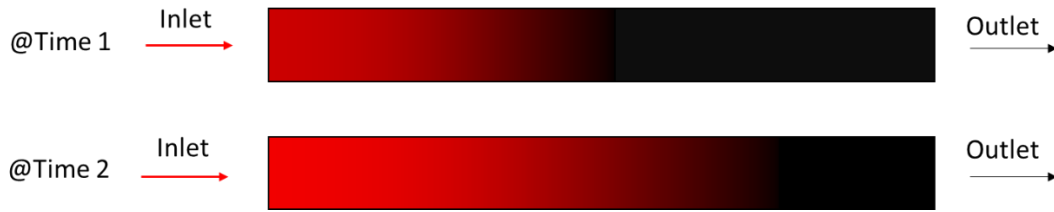
Fig. 56—Schematic diagram shows the process of first-contact miscible displacement. Red is the injected gas component, while black is the oil components.
