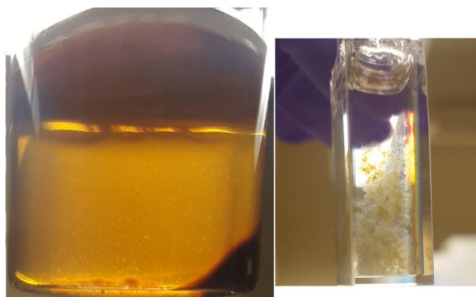
Figure 41 Cr-2 after activation in toluene (left) and after oxidation by air (right)
