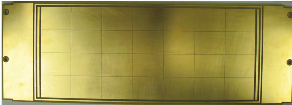
Figure 3.8: The segmented microMegas detector used in the Oxford detector.
