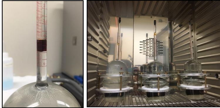
Figure 4-1 Schematic of a modified Amott cell depicting the graduated tube (left) and Amott cells inside an oven (right).
