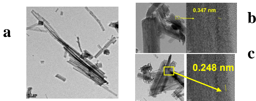
Figure 18- a) TEM image of pTNW (20h, no EtOH, st, calcination) and HRTEM and lattice fringe spacing of b) pTNW (20h, no EtOH, st, calcination) and c) pTNW (20h, no EtOH, no st, calcination)
