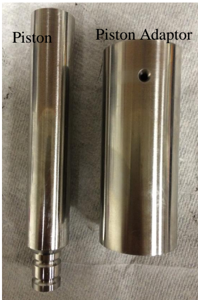
Figure 3.2 Loading system for triaxial compression tests and sample assembly setup.
