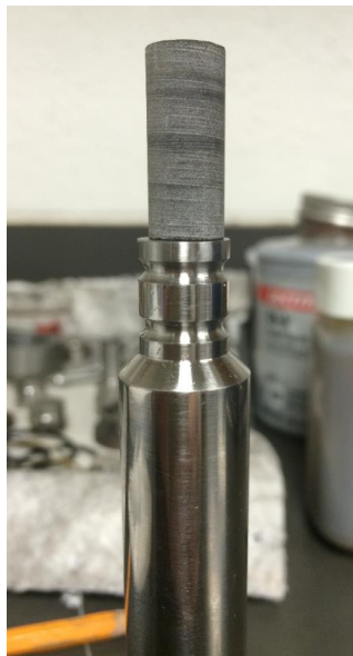
Figure 3.2 Loading system for triaxial compression tests and sample assembly setup.
