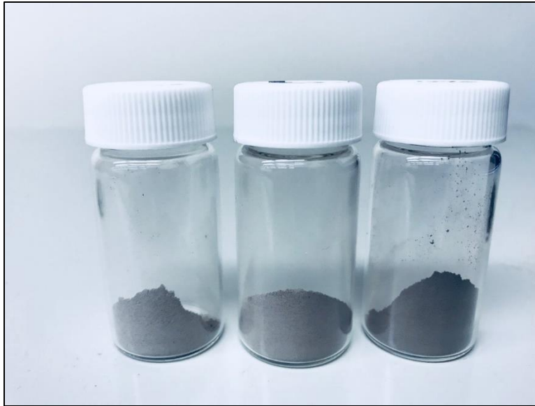
Figure 22: Zeta potential powder samples used for testing; slight color difference can be seen between the samples. In order from left to right, Core 6, 129H, 227H
