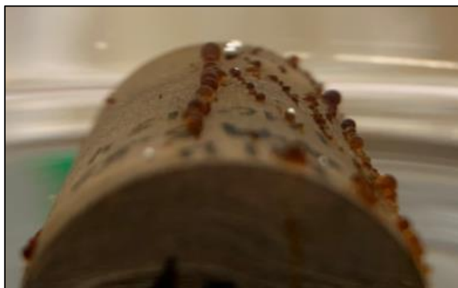
Figure 28: Core 41H 24 hours after imbibition in surfactant 2-A using 1 gpt of 2-A #4 only @ 170 °F. Looking closely you can see that the oil droplets are larger in diameter than core 38H in the figure above.
