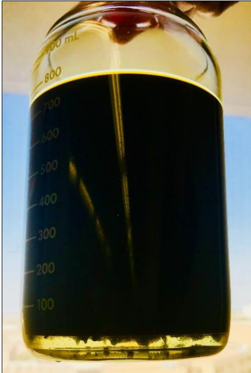
Figure 4: Picture of crude oil showing produced water and other solids.
