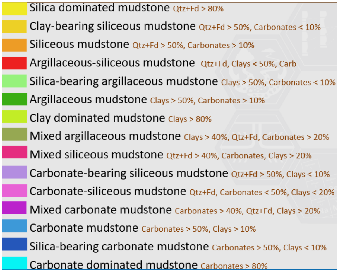
Figure 6: Color-coded chart for facies diagram found in Section 2.1.2 explaining what each color represents.
