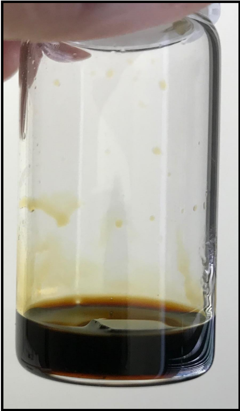
Figure 7: Example of aging process, rock chip in vial submerged in crude oil.
