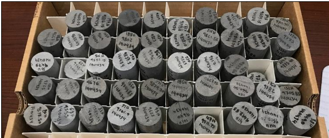
Figure 8: Photograph of core plugs provided by Marathon Oil Company.
