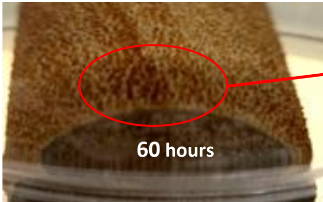
Pictures of plug 38H imbibing in surfactant 2-A (#3+#4) at 1 gpt. Oil bubbles cover the entire plug surface but are small in diameter.
