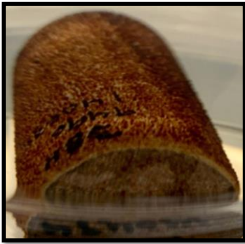
Figure 19: Core 38H in 1 gpt of 2-A after 260 hours, oil bubbles cover the entire surface but a denser streak of oil can be seen on the right-side of the core as well as in the CT scan image.
