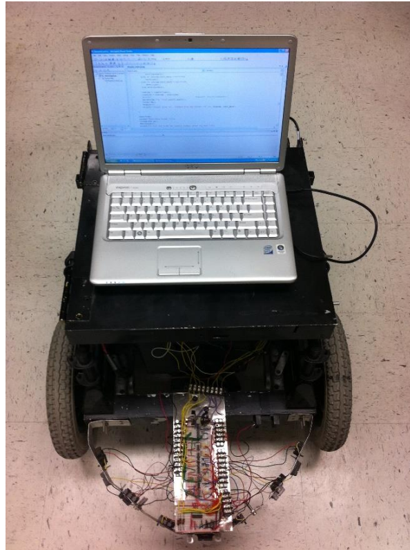
Figure 3-9. Autonomous wireless wheelchair robot
