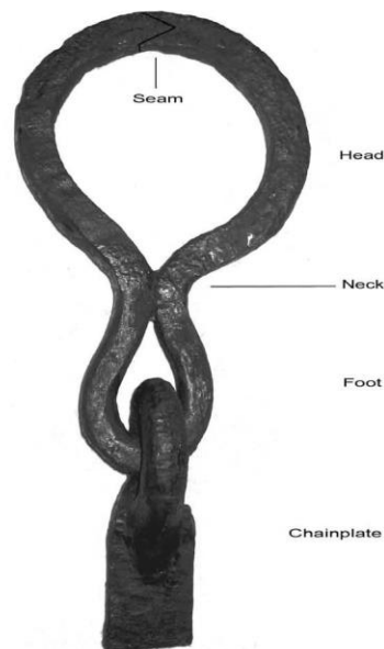
Figure 3: Chain plate # 1586 from La Belle (1686) with standard terminology (Corder 2007, 51).
