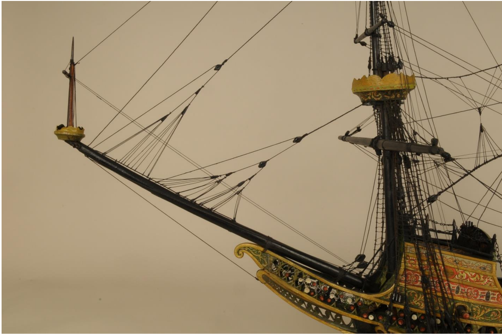
Figure 89: Portside bowsprit, yard, and rigging details of the 1593 votive model. Image from Museo Naval de Madrid, N° inventario: MNM-80.
