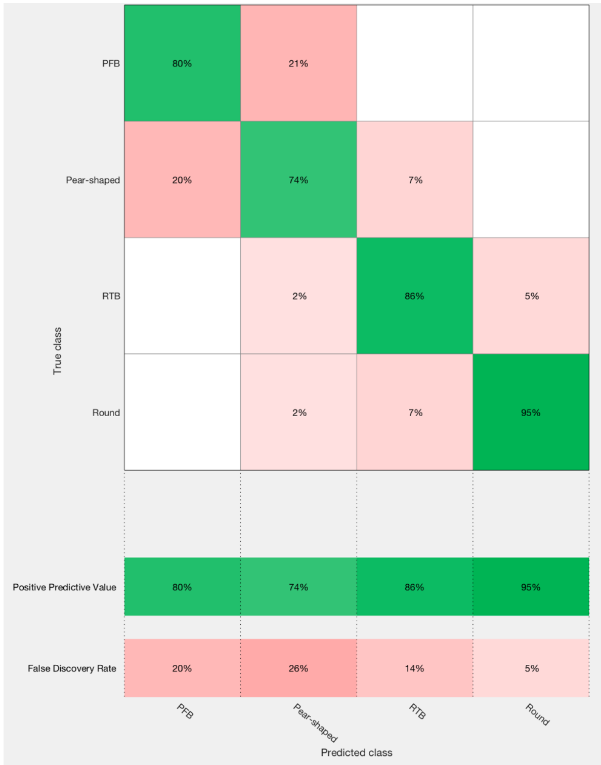
Figure 63: Model 19 Confusion Matrix. Correct predictions are shown in green, whereas incorrect predictions are in red (Image by Hannah C. Clark).
