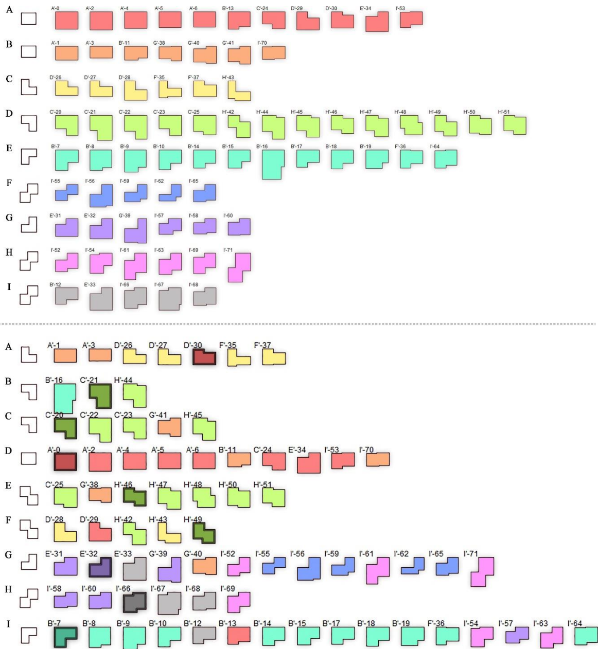
Figure 4-18. Above: the clustering subsets of the 64 cell-packing-scenario re-illustrated as a reference set; below: the clustering results of the 36 cell-packing-scenario re-illustrated according to the 64 cells with new color-coding.
