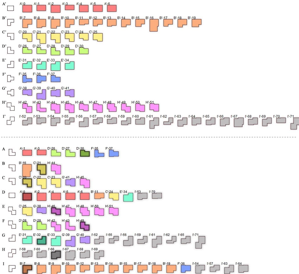
Figure 4-15. Above: the reference set; below: the clustering results of the 72 shapes using 36 cells packing, and the medoid of each cluster represented in a darker tone.
