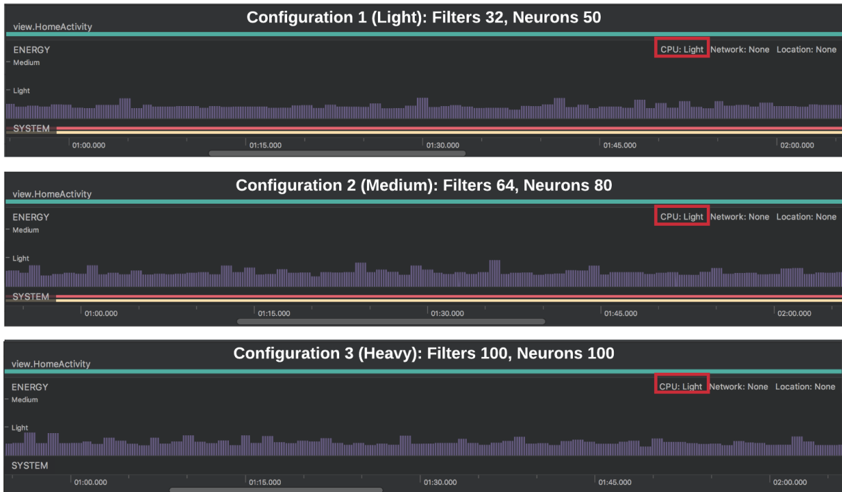
Figure 5.10: The figure shows energy consumption when running our data collection app in the smartwatch while running inferences with different hyperparameter configuration settings identified as low, medium, and heavy referring to the final number of parameters each trained model will have.
