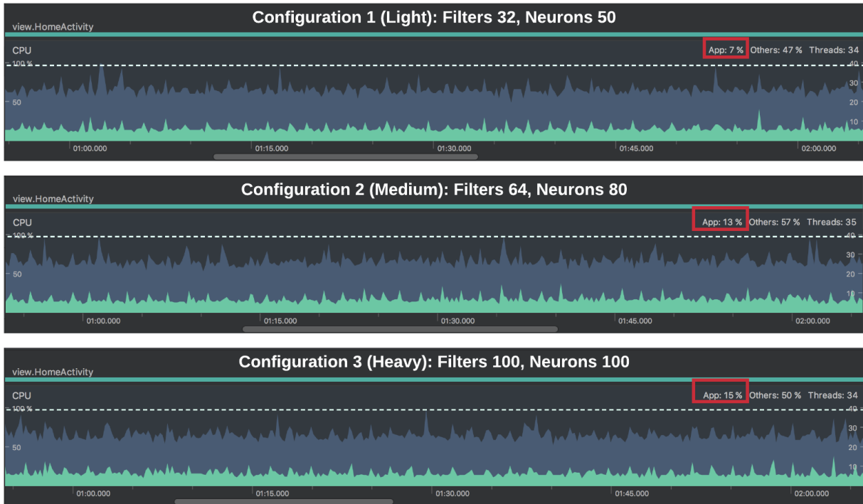
Figure 5.9: The figure shows CPU consumption when running our data collection app in the smartwatch while running inferences with different hyperparameter configuration settings identified as low, medium, and heavy referring to the final number of parameters each trained model will have. We notice a clear trend on the CPU usage as it increases as the number of parameters increases, which correlates to the hyperparameter configuration.
