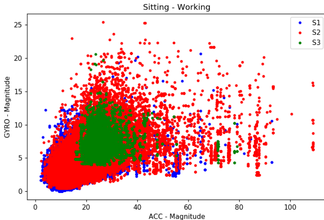
Figure 5.3: The figure shows the magnitude of accelerometer and gyroscope data corresponding to the activity sitting while working. Three subjects are shown in this figure. We can see that despite subject 1 and subject 2 seemed to share similar patterns, subject 3 seems to be clearly different and has its own patterns. This visualization suggests that users might perform activities differently.
