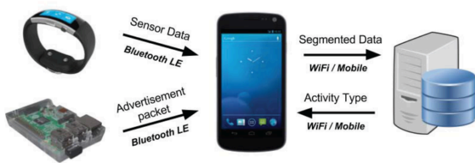
Figure 2.1: Data collection platform with BLE for micro-location. Reprinted from: [23]
