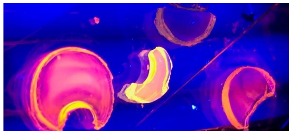
Figure 7: Cured nanocomposites showing the effect of curing conditions on sample fluorescence.
