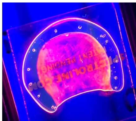
Figure 17: Resin nanocomposite over a black light to show the presence of concentration gradients.
