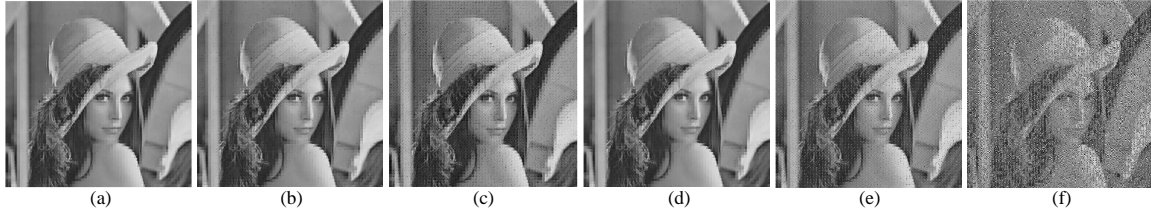
Figure 2.27: Comparison of image lenna: (a) accurate adder; (b) SARA4; (c) SARA8; (d) SARA4-DAR2; (e) GDA; (f) RAP-CLA.
