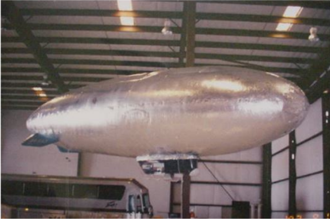
Figure 1.11: Cycloidal rotor powered Blimp [51].
