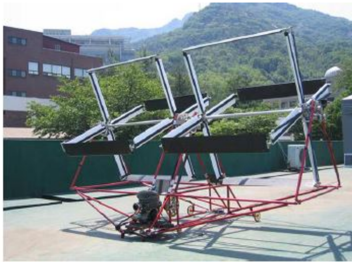
Figure 1.15: 46 kg cycloidal rotor based UAV built by Yun et al. [63].
