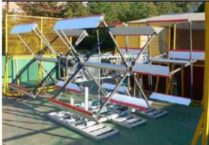
Figure 1.16: 100 kg quad-cyclocopter built by Hwang et al. [66].
