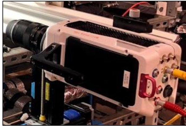
Figure 21. High-speed camera (Phantom V711)
