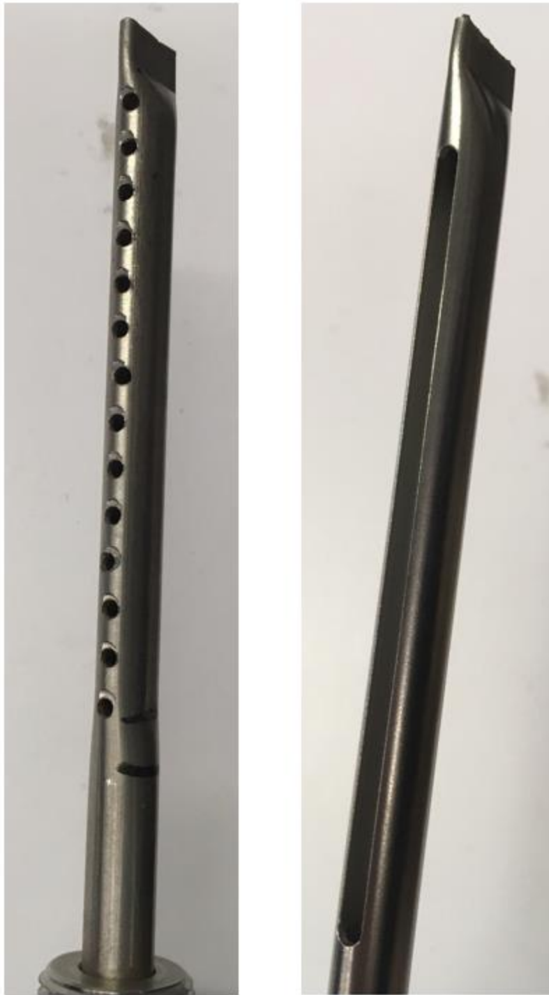
Figure 5.5. The first and second versions of the NO injection pipe used for the ACE facility
