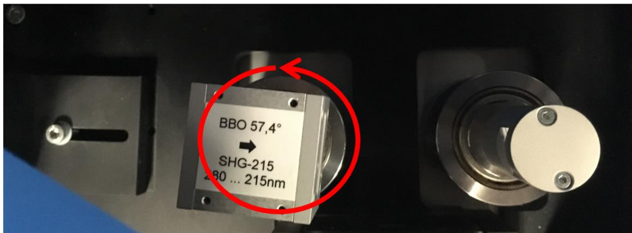
Figure 2.4. An image of the BBO contained in the FCU of the laser system. The red arrow signifies where the stepper motor is changing positions as the motor position is scanned.
