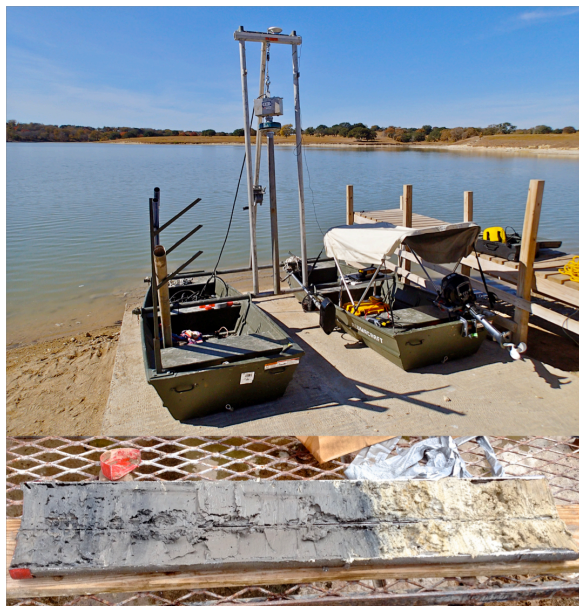
1 2 Figure 4. Reservoir sediment coring apparatus (top) and representative sediment profile 3 (bottom). 4
