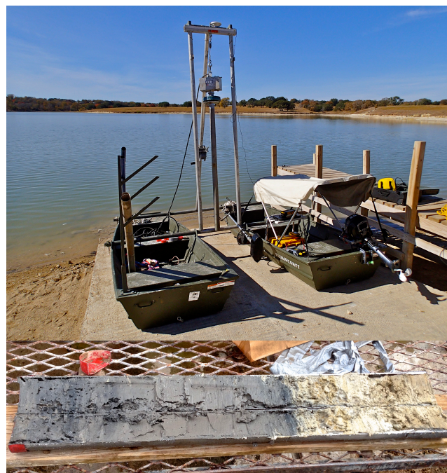
Figure 4. Reservoir sediment coring apparatus (top) and representative sediment profile (bottom).
