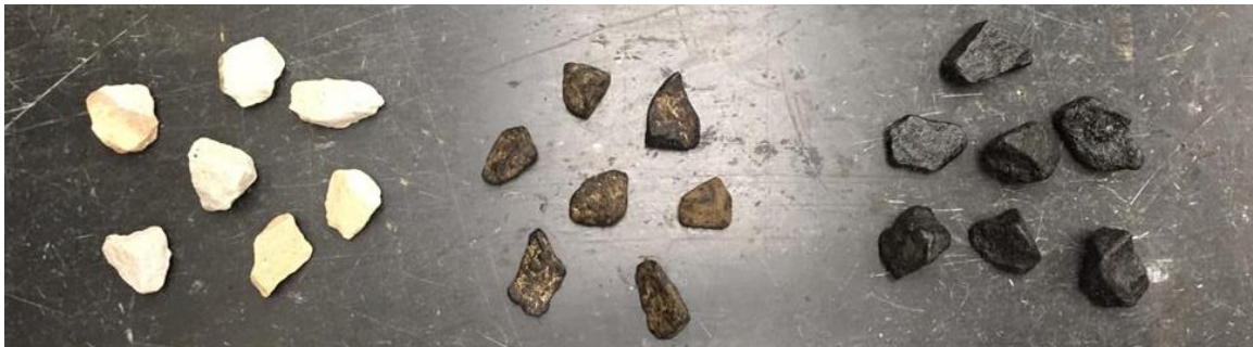
Figure 14. Coatability for a 0.5 RBR mixture with various recycling agent incorporation methods: virgin aggregate (left), aggregates after replacing the substitute binder by the full recycling agent amount (middle), and aggregates with no replacement of the substitute binder (right).
