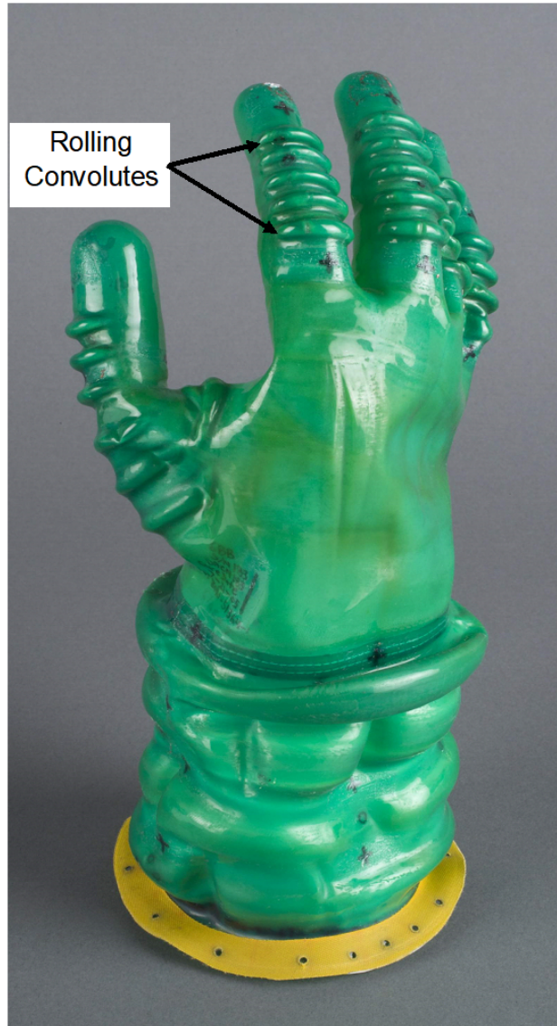
Figure 1.11: EVA Glove Pressure Bladder Convolutates
