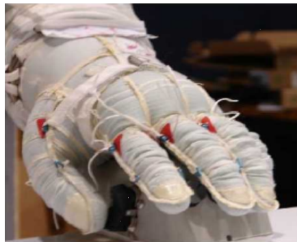
Figure 1.9: EVA Glove Restraint Layer [17]
