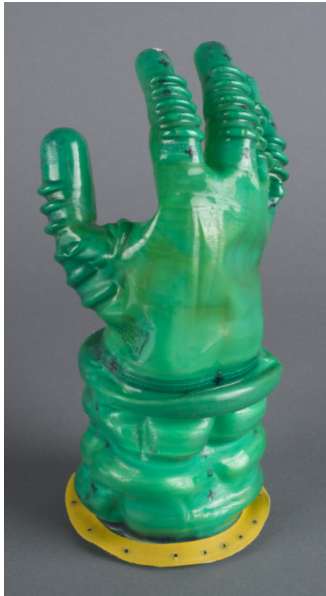
Figure 1.8: EVA Glove Pressure Bladder [16]
