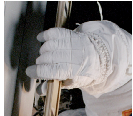
Figure 1.10: EVA Glove Thermal Micrometeoroid Garment [13]
