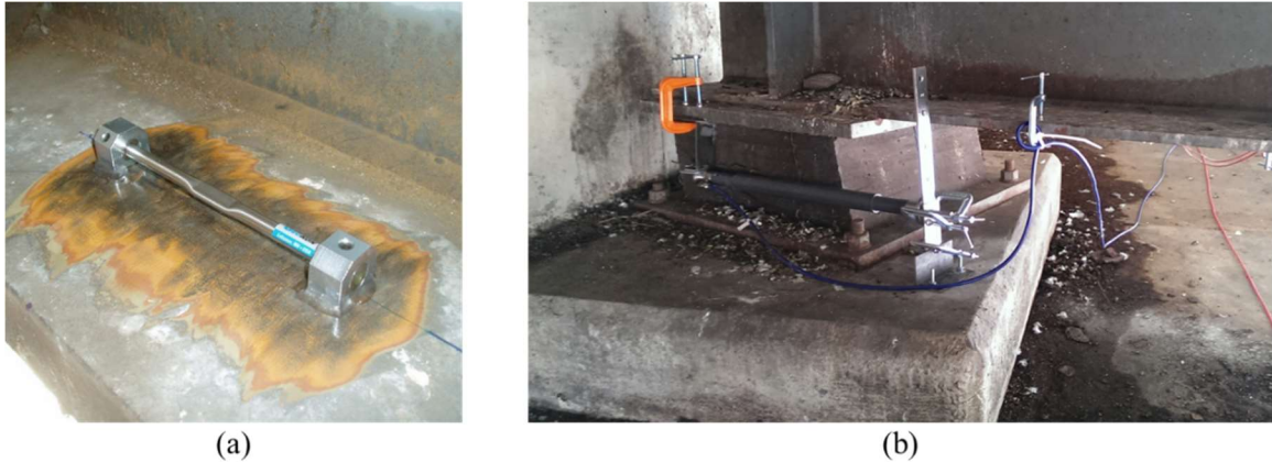
Figure 30: Sensing Equipment: a) Strain Gage and b) Displacement Gage (Reprinted from Murphy and Yarnold 2018)
