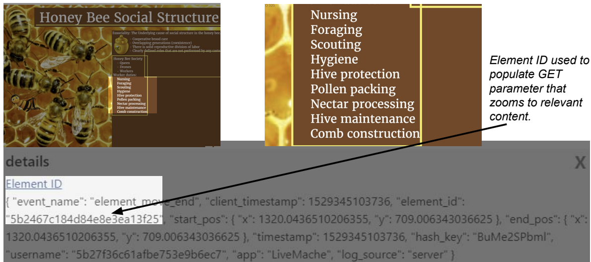
Figure 4.22: An example from LiveMache where the Detail Window includes a link that zooms to the correct curation at the relevant region.
