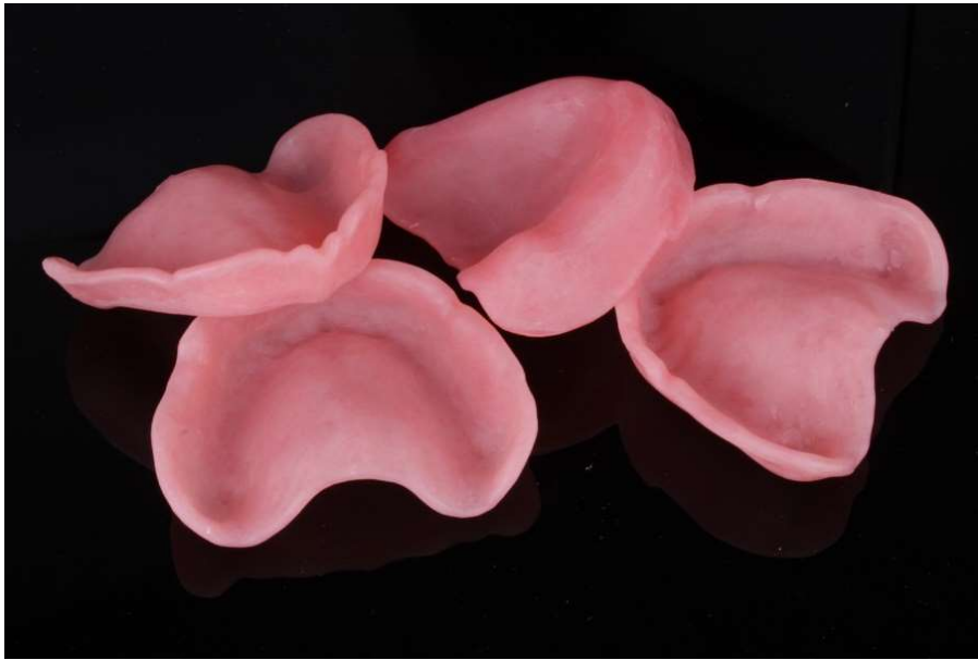
Figure 4. Milled record base specimens.
