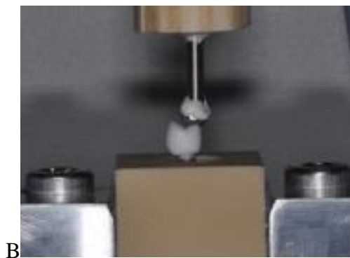
Figure 14 A: The milled Co-Cr stainless steel crown for mandibular lower second premolar with proper design and in occlusion with AM zirconia crown. B: The assembly of loading arm which was mounted onto the loading frame of the Universal Testing Machine before final repositioning of the sample.
