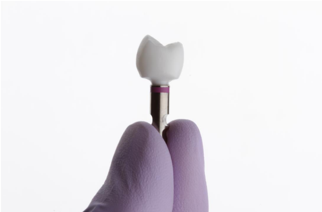
Figure 12 AM full contour monolithic zirconia cemented on zirconia abutment before mechanical testing.
