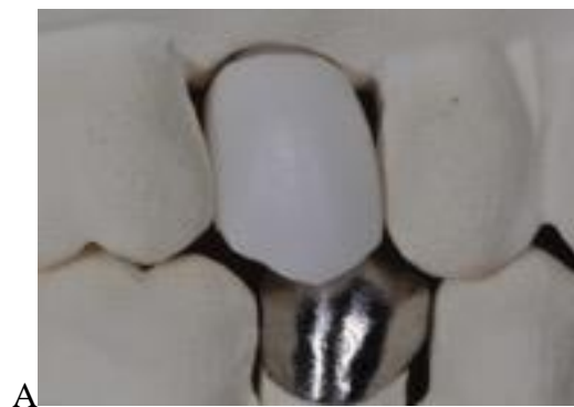
Figure 14 A: The milled Co-Cr stainless steel crown for mandibular lower second premolar with proper design and in occlusion with AM zirconia crown. B: The assembly of loading arm which was mounted onto the loading frame of the Universal Testing Machine before final repositioning of the sample.
