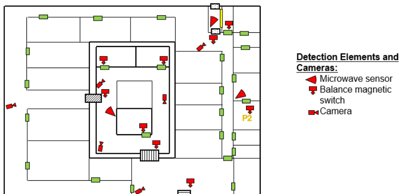
Figure 79. Detailed Schematic of Detection Elements in Building Interior Reprinted with Permission from 22 .
