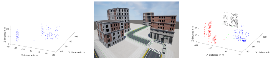
Figure 4.8: Results of NBMV planner applied to a bigger environment. Initial map on left, final map on right. Middle shows original structure. Reprinted from Vemprala and Saripalli 66
