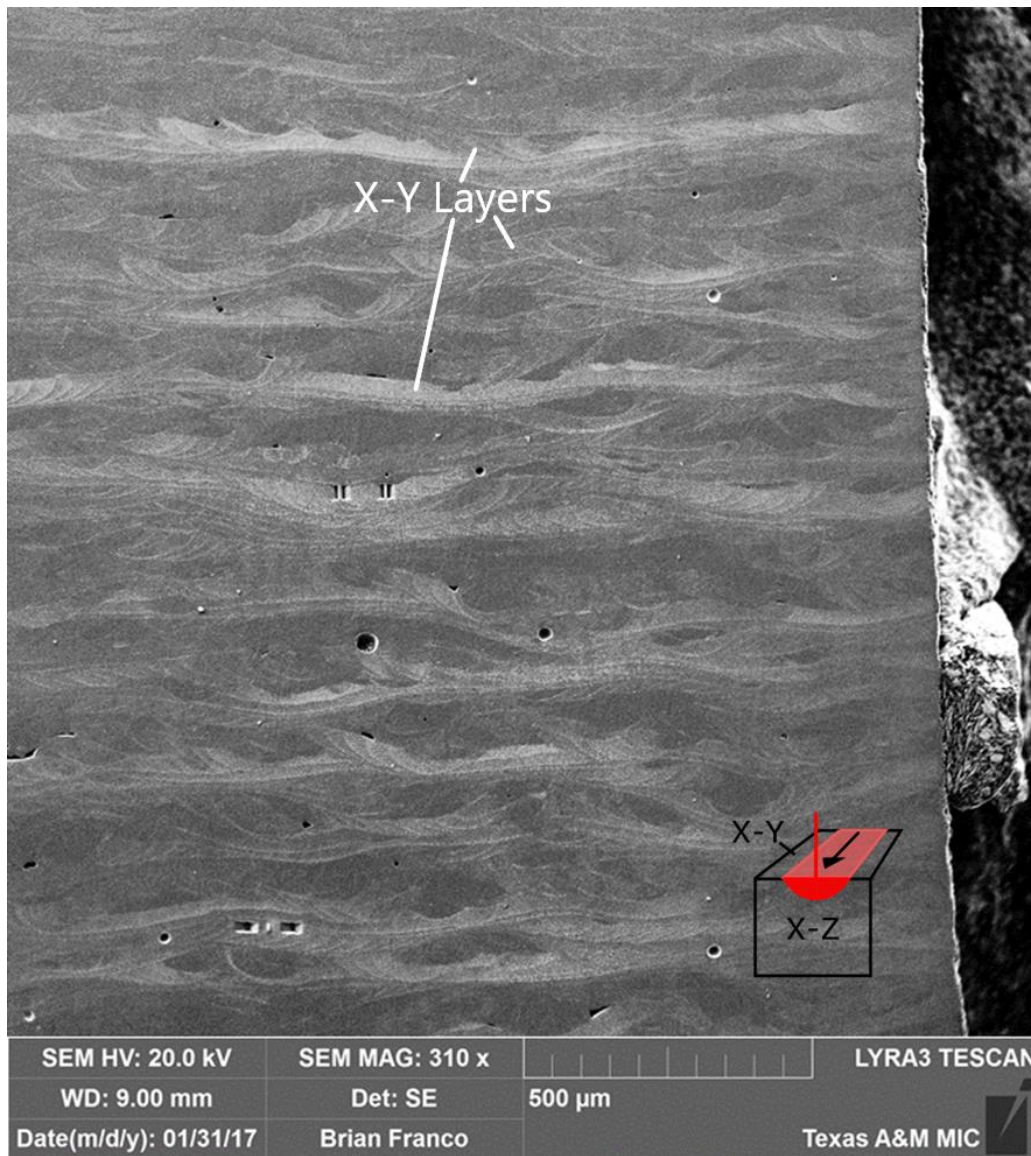
Figure 42: Polished and etched X-Z plane of the H35 cube. Individual X-Y layers, as well as single melt tracks can be seen.
