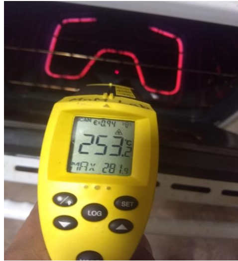
Figure 47 Non-contact type of temperature measurement using IR gun
