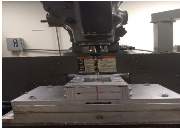
Figure 25 Hole drilling operation in the clamped stationary plate using a twist drill
