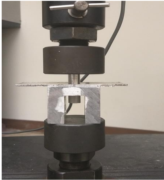
Figure 48 Shear test of Shrink fit assembly
