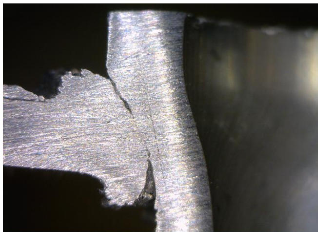
Figure 39 Microscopic image of the joint formed at spindle speed 1500 rpm, feed rate 2.116 mm/s, interference 0.635 mm, plate thickness 2 mm
