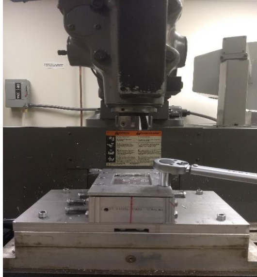
Figure 17 Torque applied to Fixture bolts
