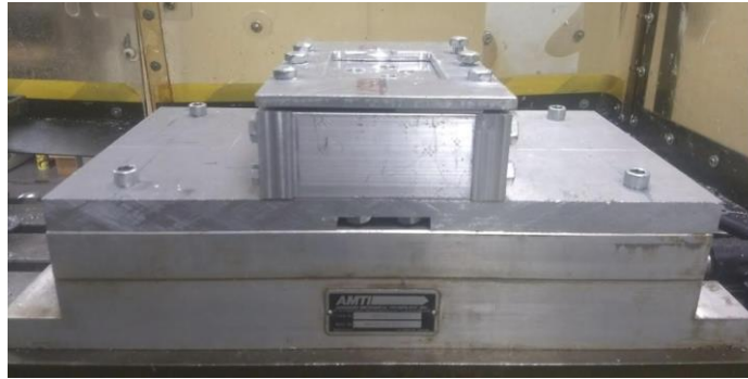
Figure 12 Fixture fastened to table mounted dynamometer
