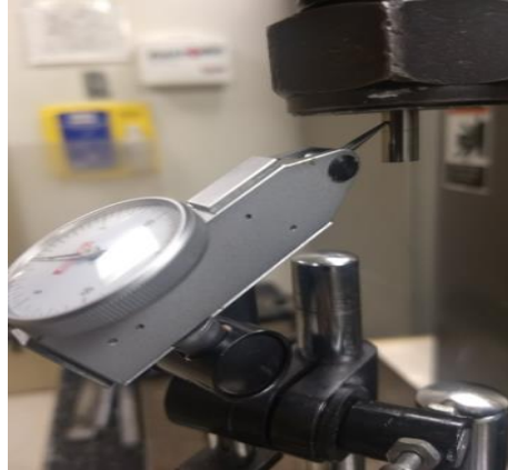
Figure 10 Run-out error measurement of machine spindle with a dial gauge
