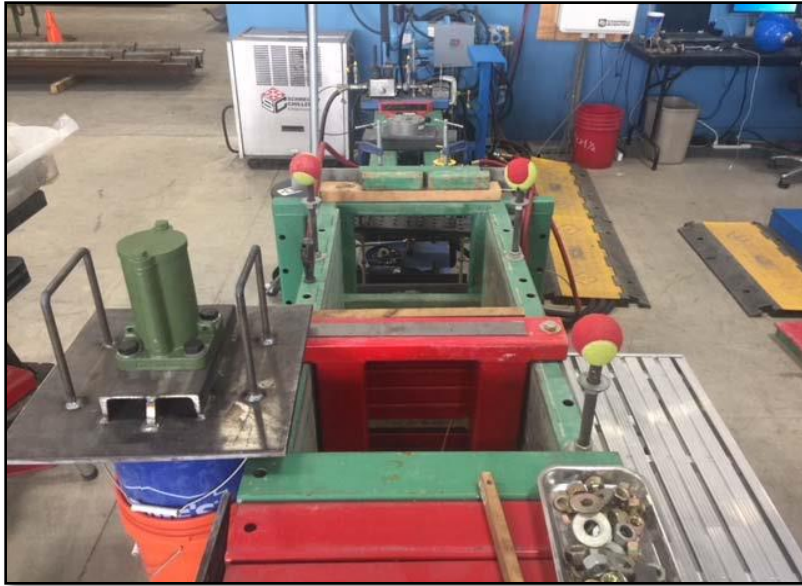
Figure 3-13. Pullout Test Apparatus (Taylor, 2018)
