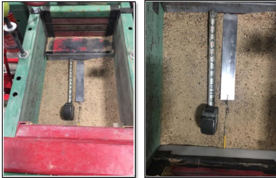
Figure 4-52. Placement of Soil-Reinforcing in Soil-Box
