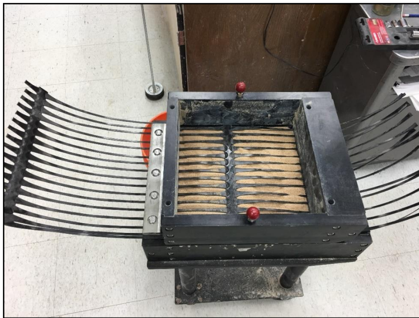
Figure 4-47. Interface Direct Shear Test Setup on Geogrid
