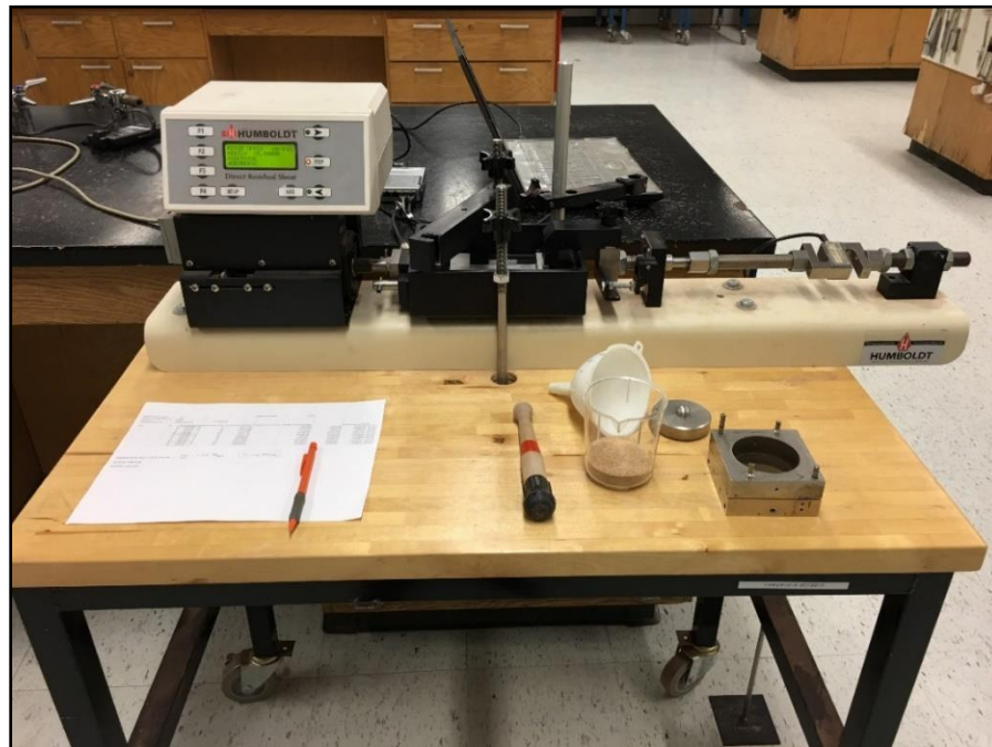
Figure 3-1. Small Direct Shear Apparatus, TAMU Laboratory
