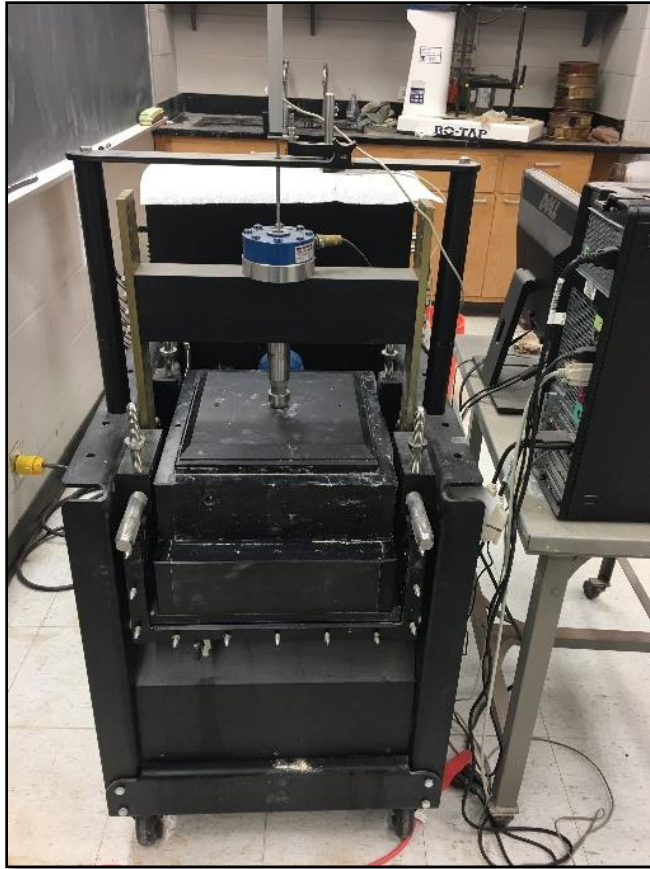
Figure 4-8. Placement of Shear Box in the Water Bath
