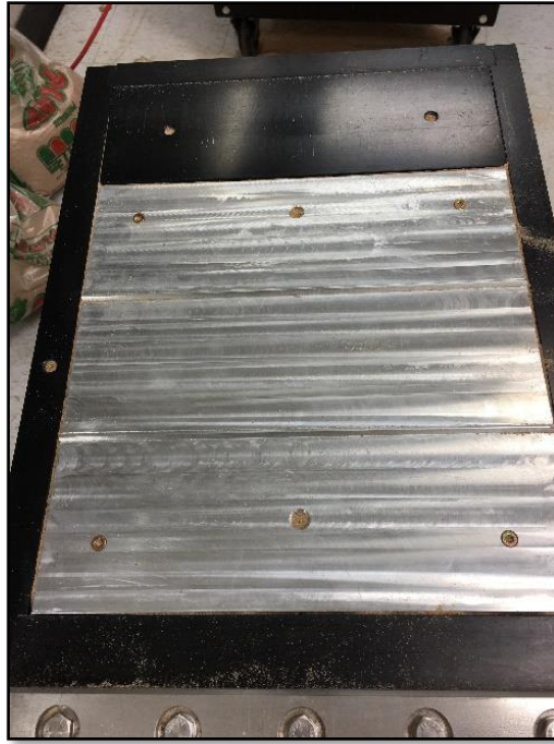
Figure 4-34. Placement of the Spacer and the Aluminum Plate inside the Lower Half of the Shear Box
