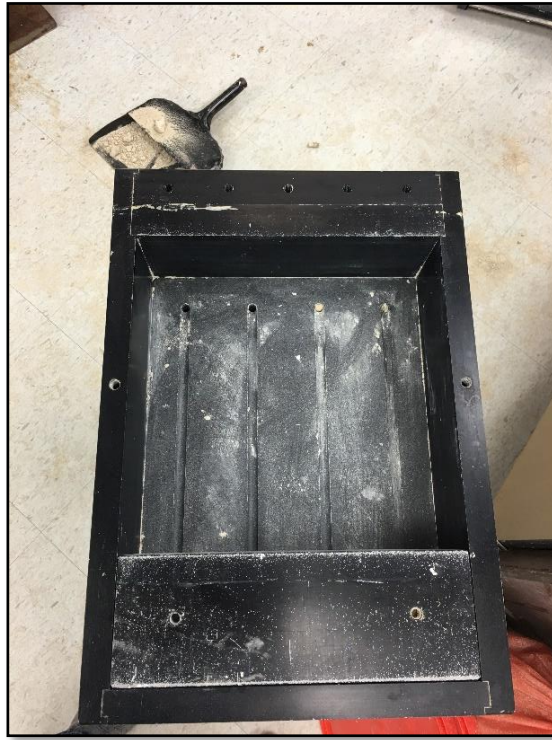
Figure 4-2. Lower Shear Box Standing on the Shear Box Stand
