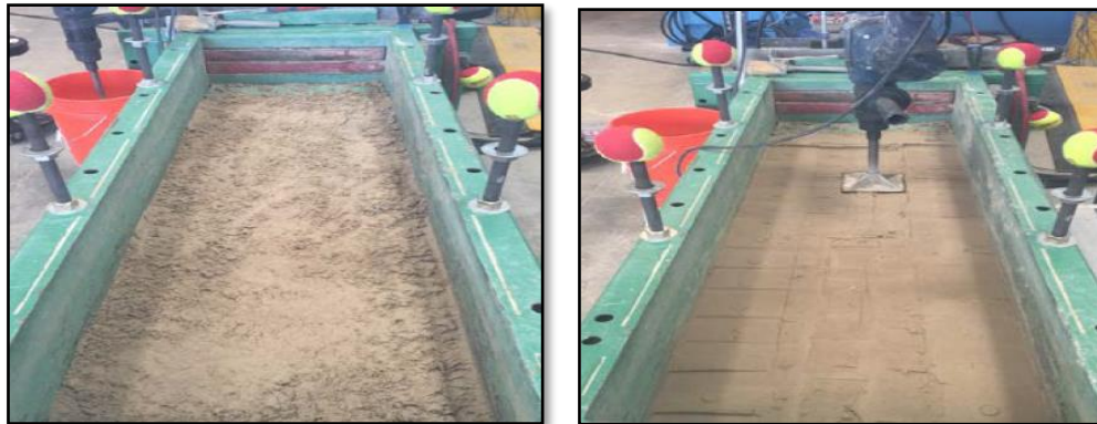
Figure 4-54.Placing and Compacting Soil
