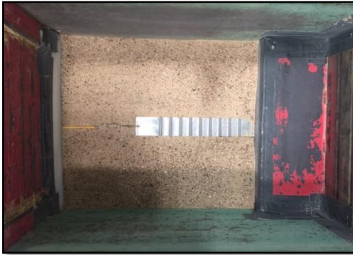
Figure 3-34. Plan View of the 9-Ribbed Steel Strip-Half Box
