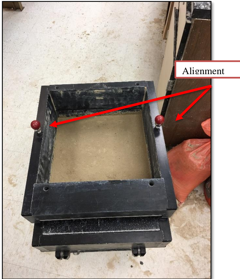
Figure 4-3. Placement of Top Shear Box and Alignment Screws
