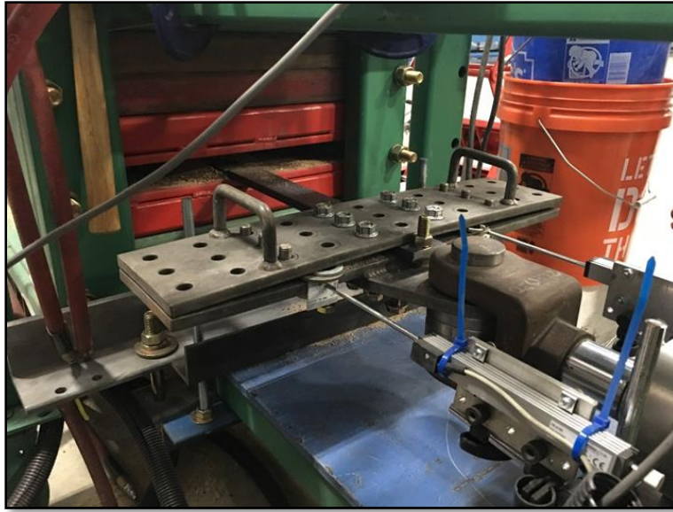
Figure 3-20. Soil-Reinforcing Clamp (Taylor, 2018)
