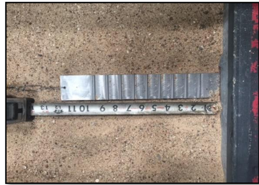
Figure 3-34. Plan View of the 9-Ribbed Steel Strip-Half Box
